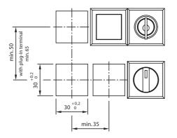
Indicator-, pushbutton-, keylock switch-, selector switch actuator short lever
