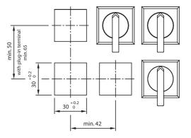
Selector switch actuator long lever
