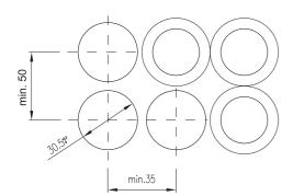
04 Long Lever Cut-outs, Flush Mounting
