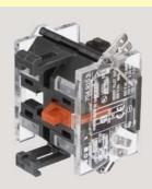
Contact block, plug-in terminal, 6.3mm, slow-make with forced opening silver contacts
