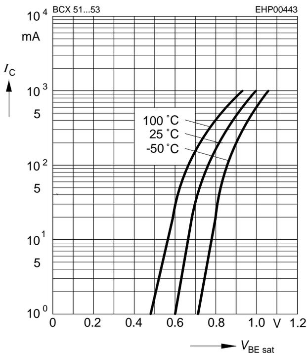
**Collector current  $I_C = f(V_{BE})$**
