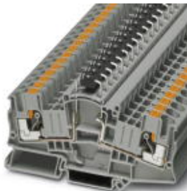
Component terminal block, Connection method: Push-in connection, Cross section: 0.5 mm 2 -10 mm 2 , AWG: 20 - 10, Width: 8.2 mm, Color: gray
