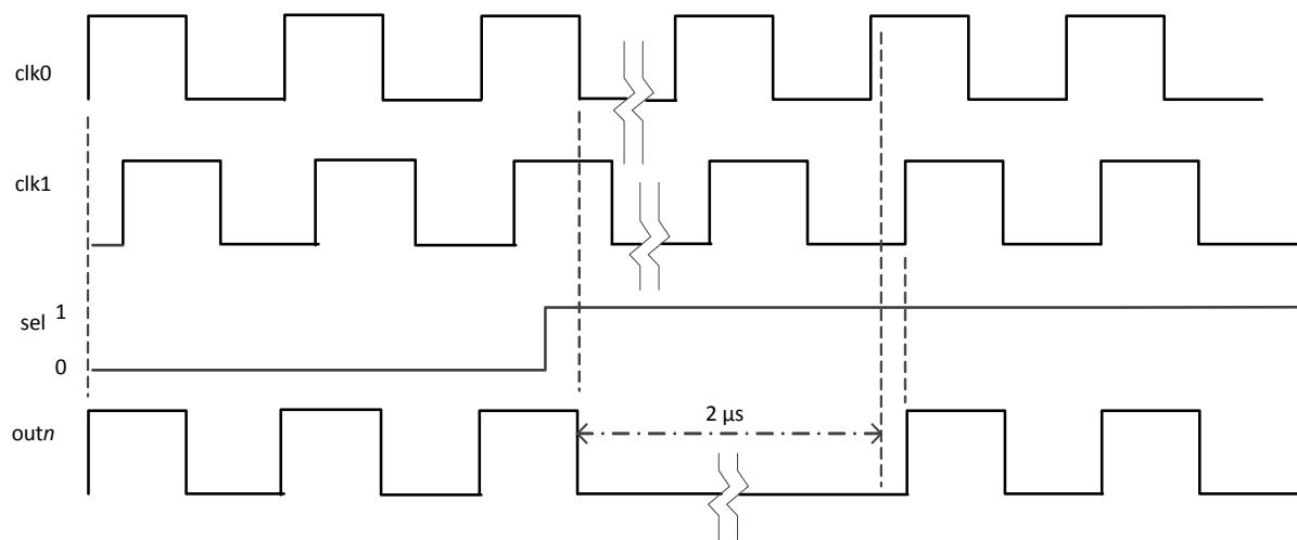
**Figure 4 - Output During Clock Switch - Both Clocks Running**
