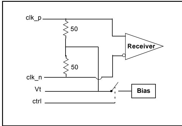
**Figure 3 - Simplified Diagram of input stage**
