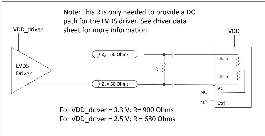
**Figure 8 - Clock Input - LVDS - AC Coupled**
