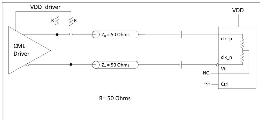
**Figure 9 - Clock Input - CML- AC Coupled**
