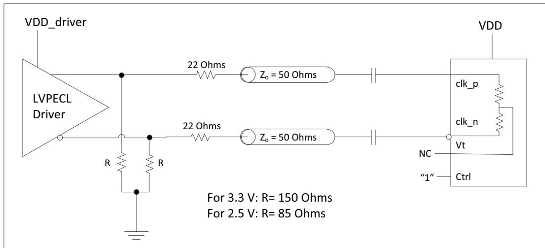
**Figure 6 - Clock Input - LVPECL - AC Coupled**
