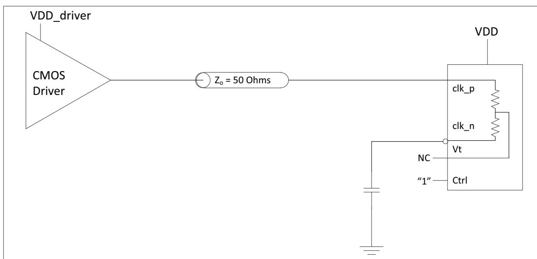
**Figure 12 - Clock Input - DC-coupled 3.3V CMOS**
