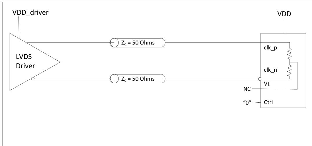
**Figure 7 - Clock Input - LVDS - DC Coupled**
