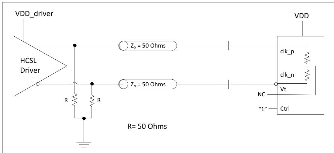
**Figure 10 - Clock Input - HCSL- AC Coupled**
