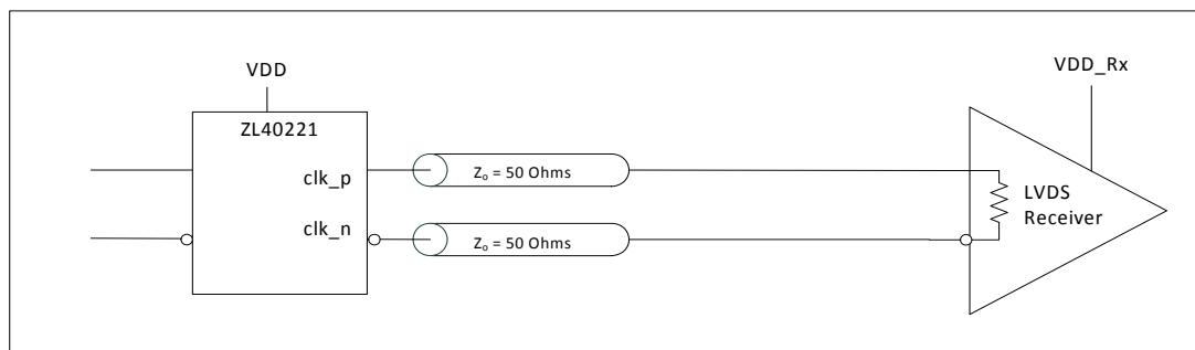
**Figure 14 - LVDS DC Coupled Termination (Internal Receiver Termination)**
