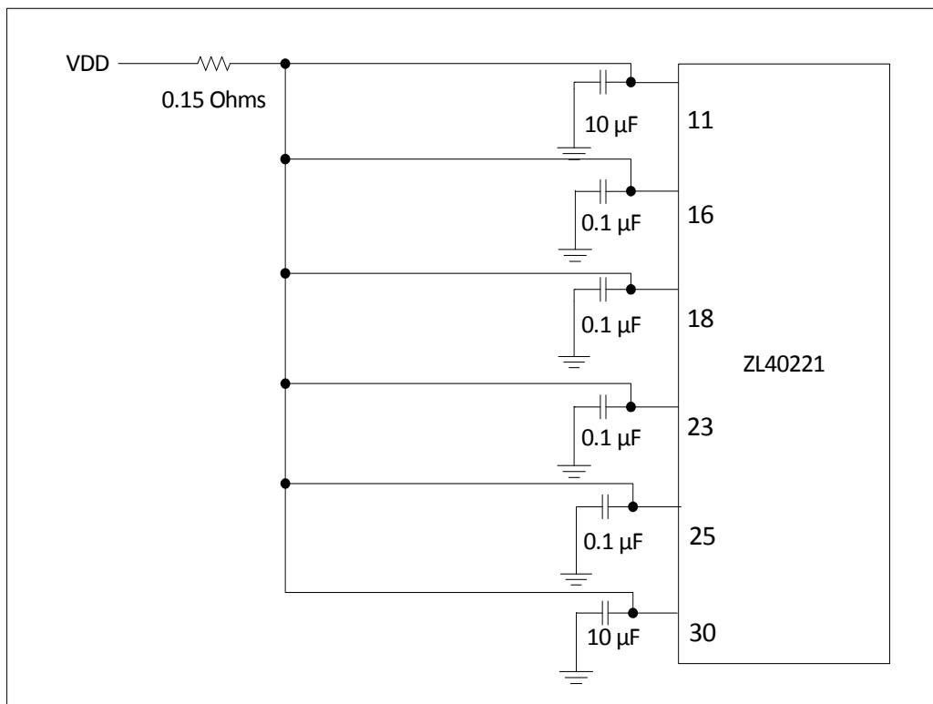
Figure 19 - Decoupling Connections for Power Pins
