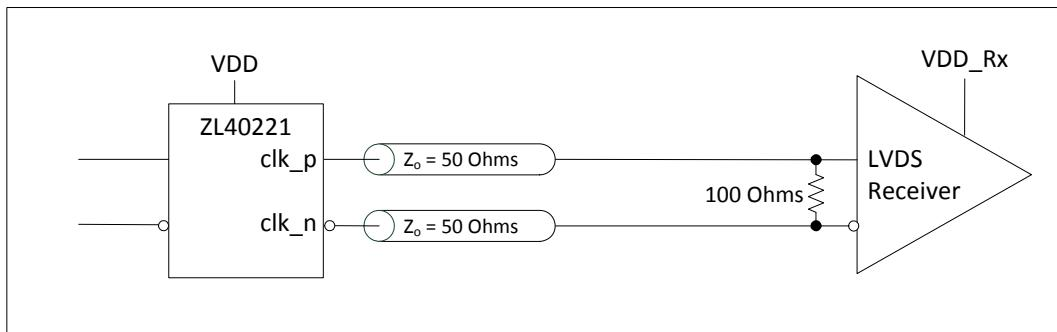
**Figure 15 - LVDS DC Coupled Termination (External Receiver Termination)**
