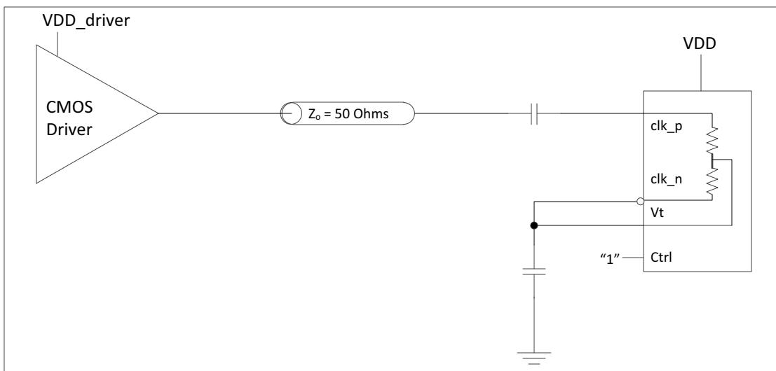
**Figure 11 - Clock Input - AC-coupled Single-Ended**
