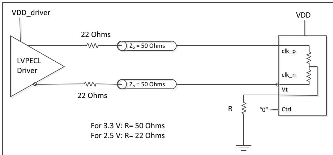
**Figure 5 - Clock Input - LVPECL - DC Coupled**
