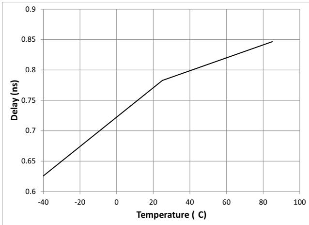
Propogation Delay versus Temperature
