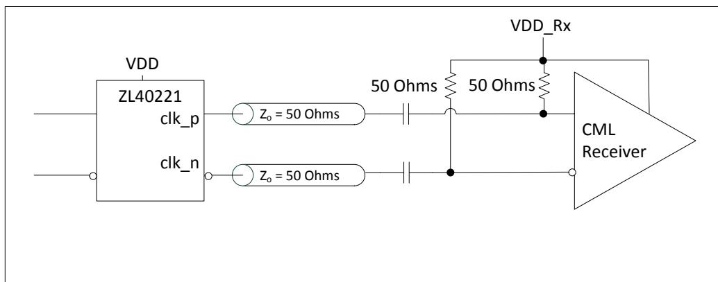
**Figure 17 - LVDS AC Output Termination for CML Inputs**
