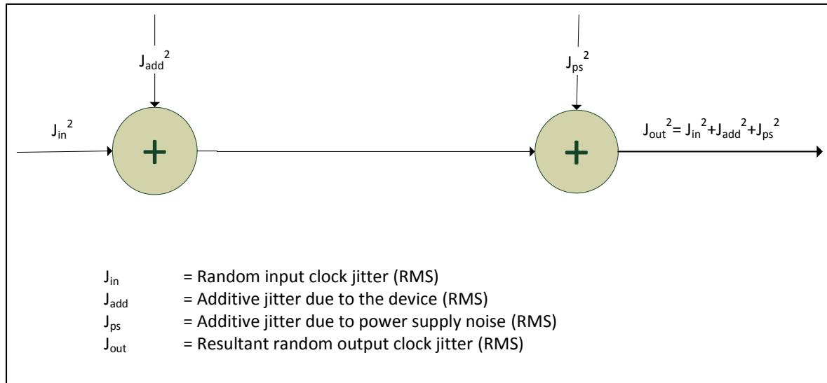
**Figure 18 - Additive Jitter**
