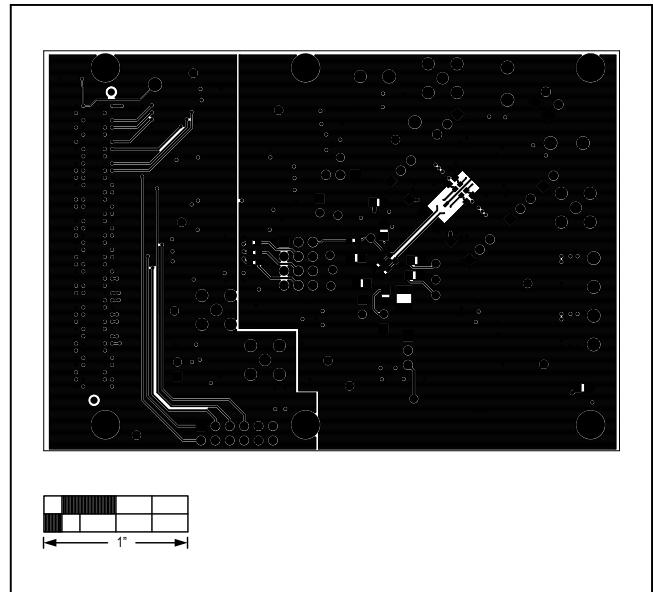
Figure 15. MAX11905 Differential EV Kit PCB Layout—Solder Side
