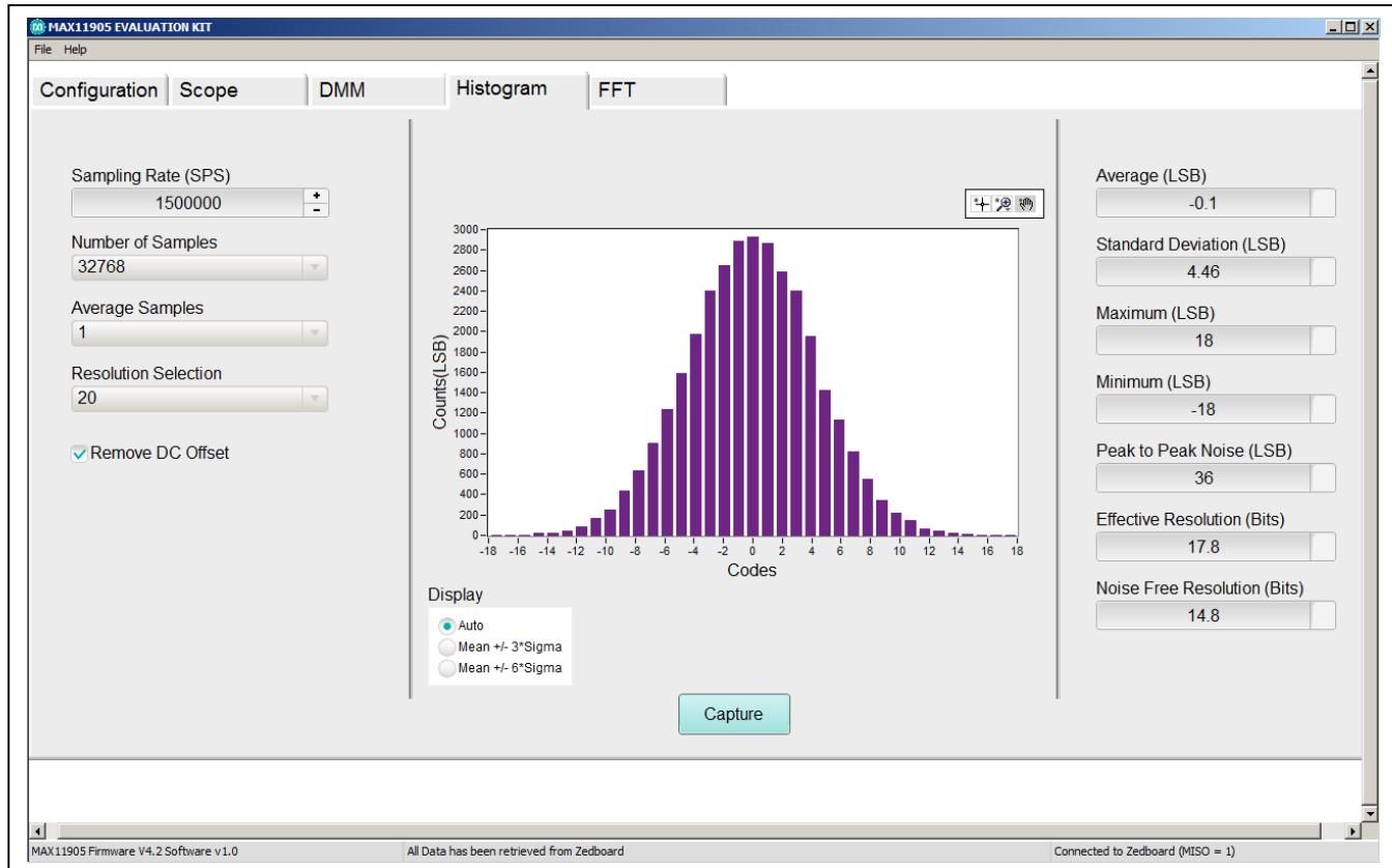
Figure 4. MAX11905 EV Kit Main Window (Histogram Tab)
