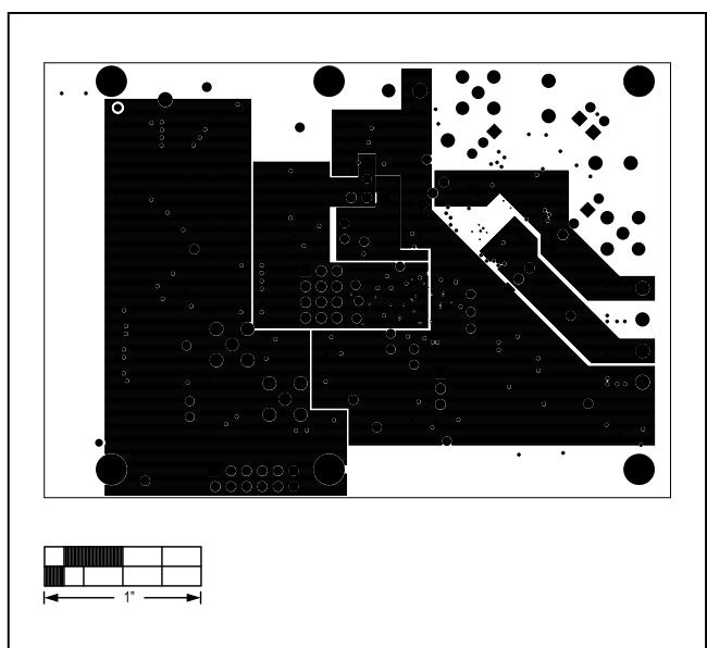
Figure 12. MAX11905 Differential EV Kit PCB Layout—Layer 3
