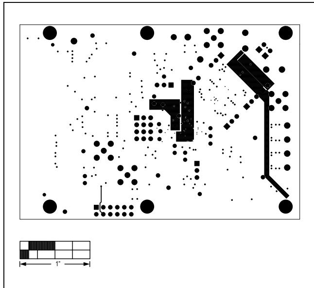
Figure 13. MAX11905 Differential EV Kit PCB Layout—Layer 4
