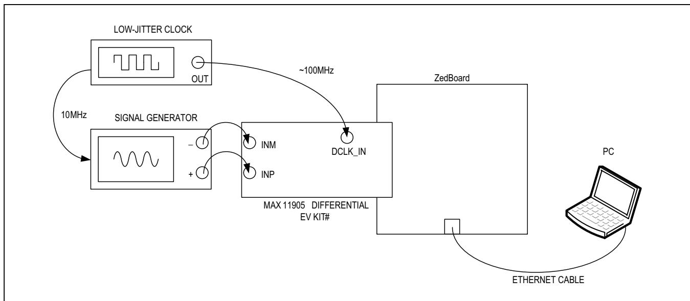
Figure 5. MAX11905 Differential EV Kit Coherent Sampling Setup
