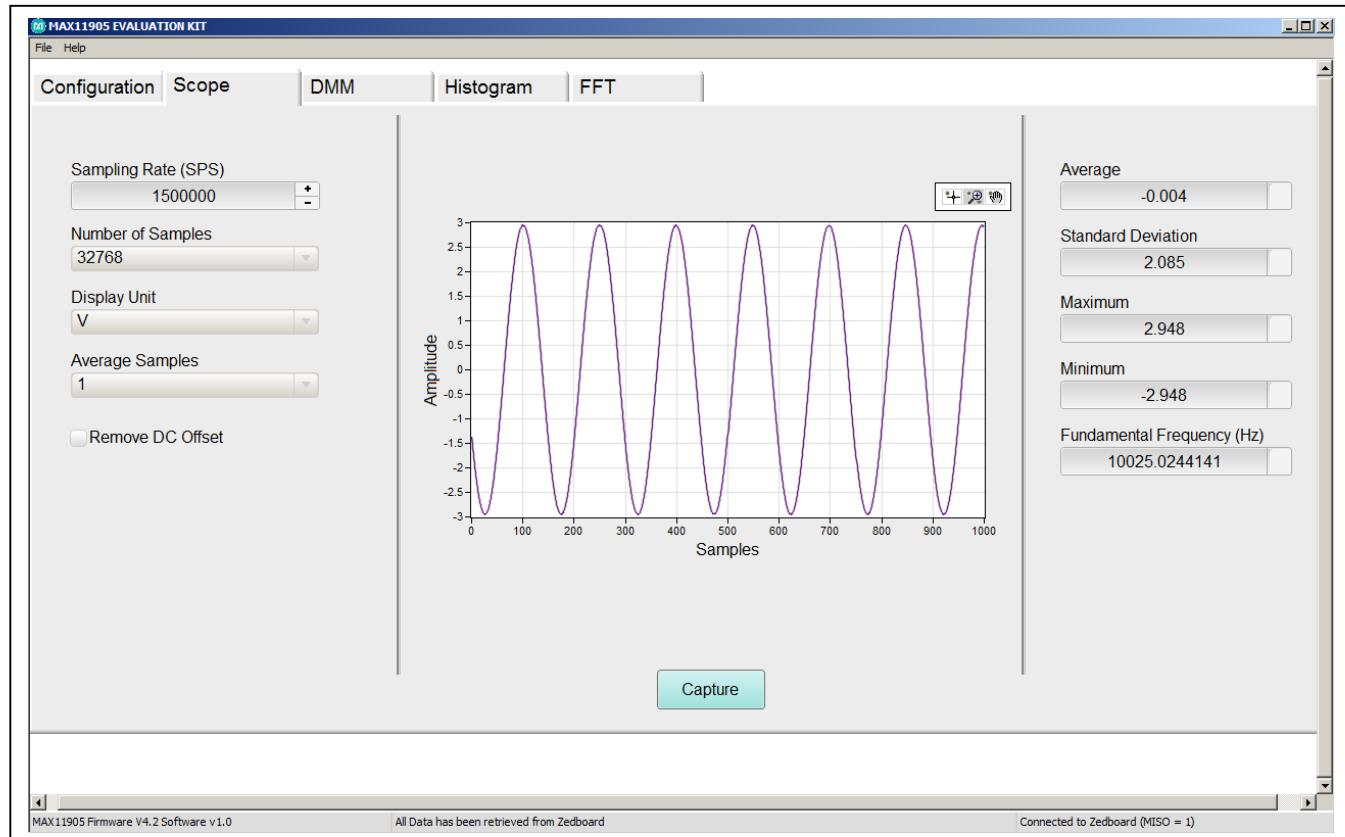
Figure 2. MAX11905 EV Kit Main Window (Scope Tab)
