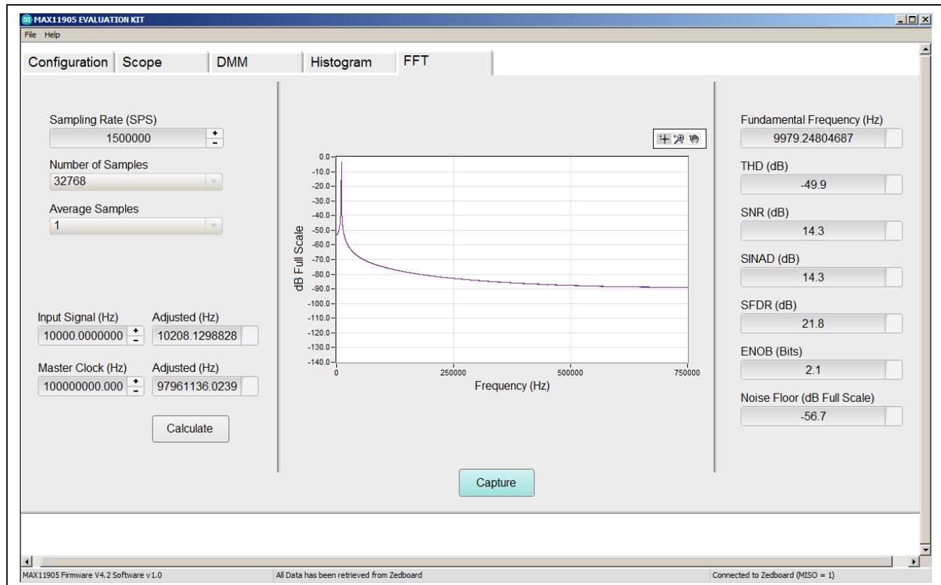
Figure 7. MAX11905 EV Kit Main Window, Noncoherent Sampling Results (FFT Tab)
