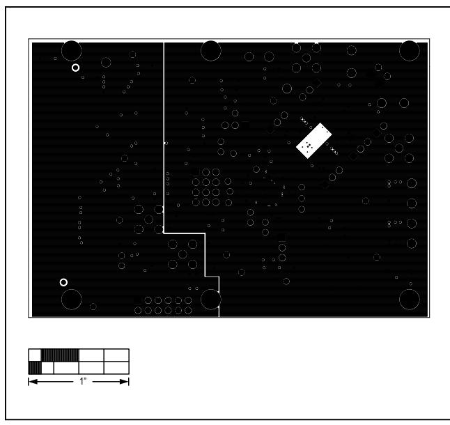
Figure 14. MAX11905 Differential EV Kit PCB Layout—Layer 5
