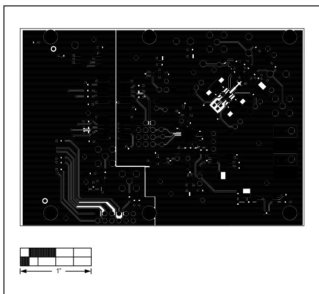
Figure 10. MAX11905 Differential EV Kit PCB Layout—Component Side
