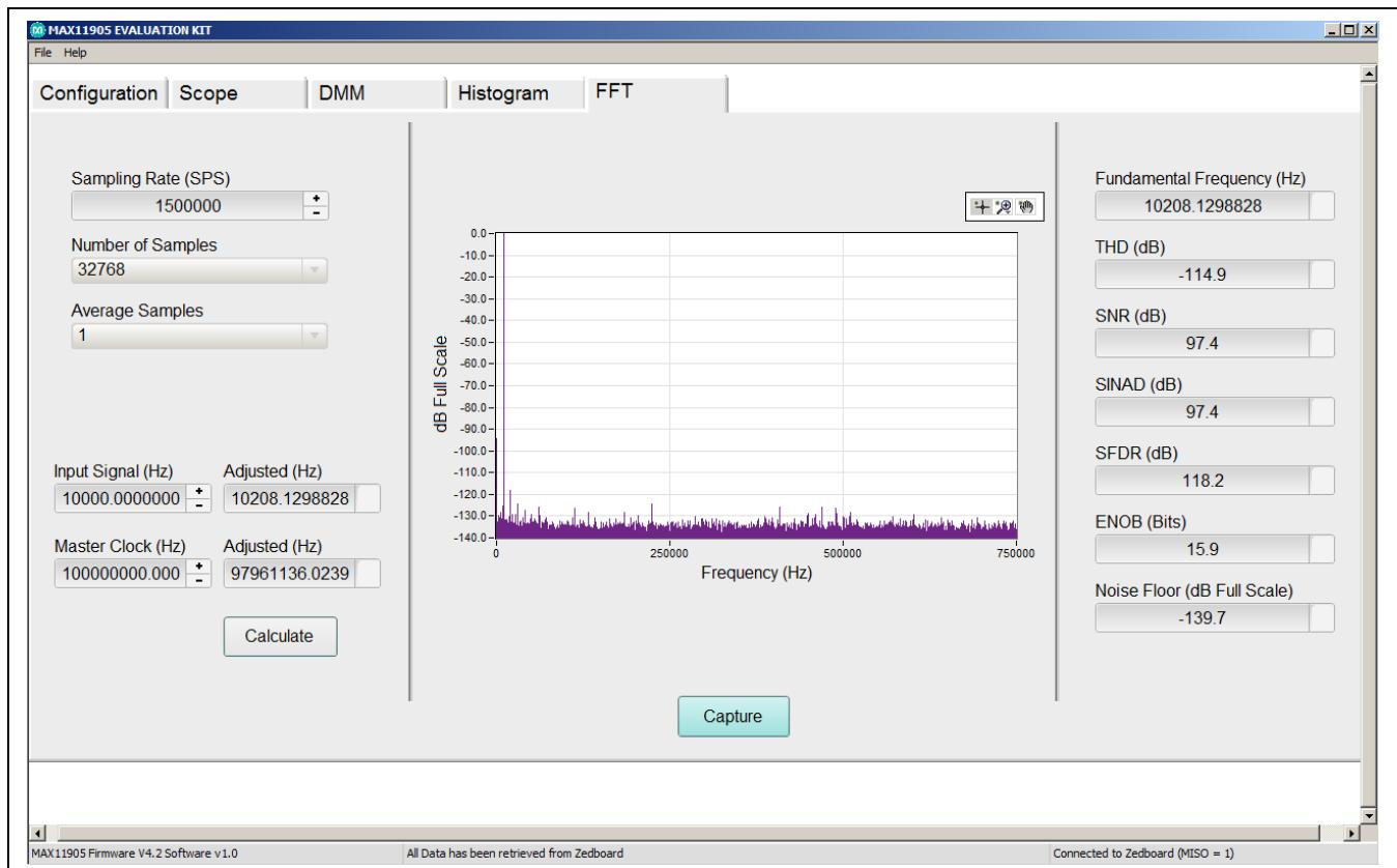
Figure 6. MAX11905 EV Kit Main Window, Coherent Sampling Results (FFT Tab)
