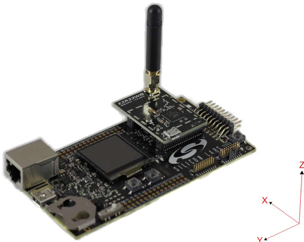
Figure 6.2. DUT: BRD4505B (Rev. A00) Radio Board with Wireless Starter Kit Mainboard
