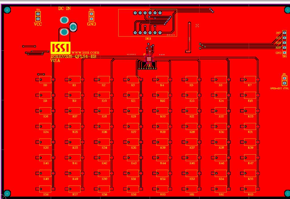
Figure 4: Board PCB Layout- Top Layer
