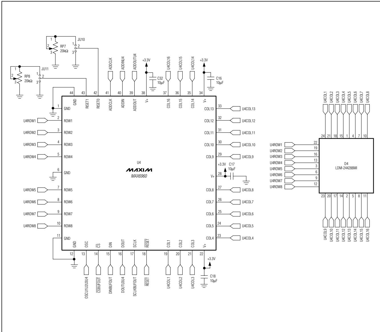
Figure 5. MAX6960 EV Kit Schematic (Sheet 4 of 6)
