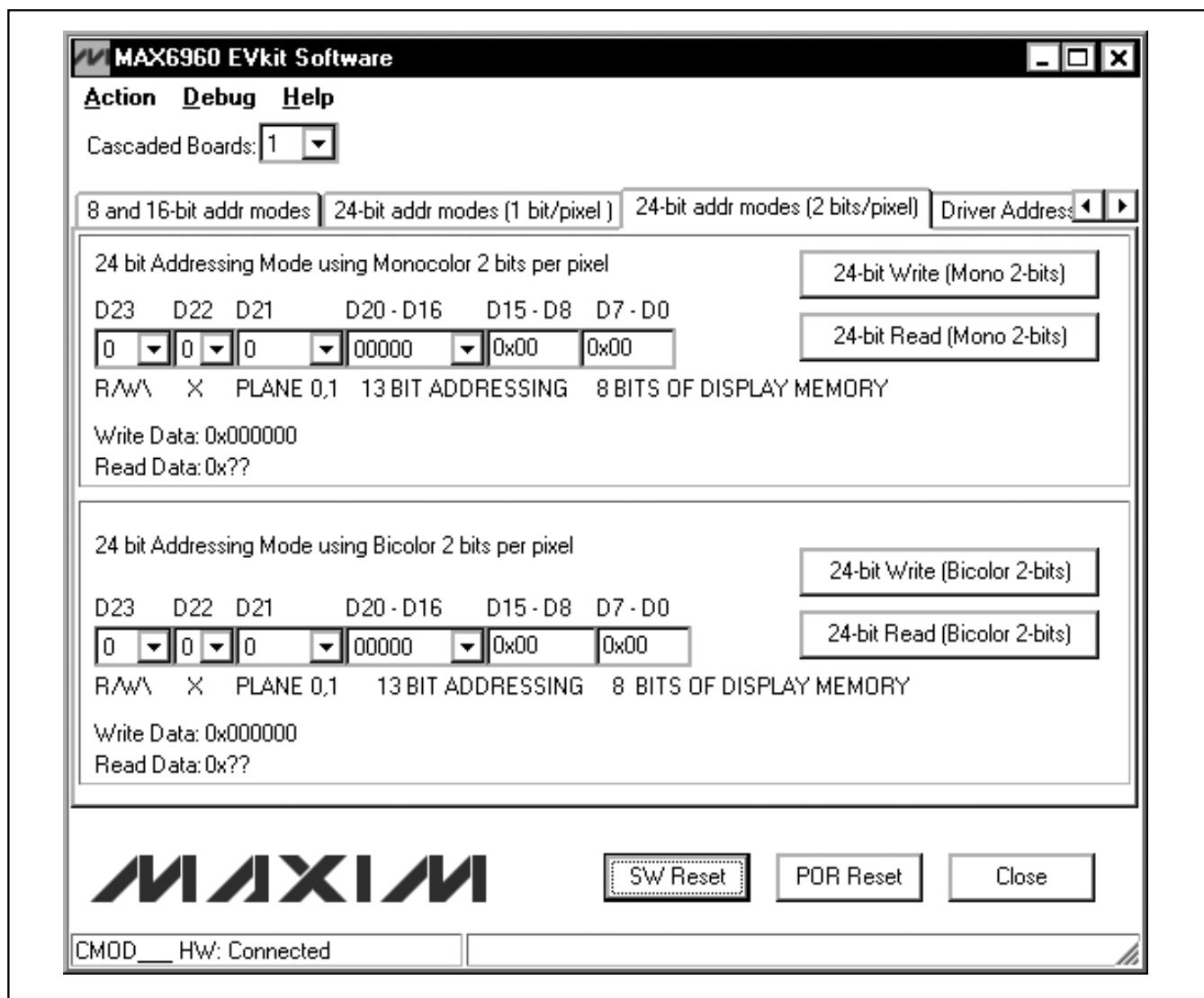
Figure 3. 24-Bit Addressing Modes (2 Bits/Pixel) Tab
