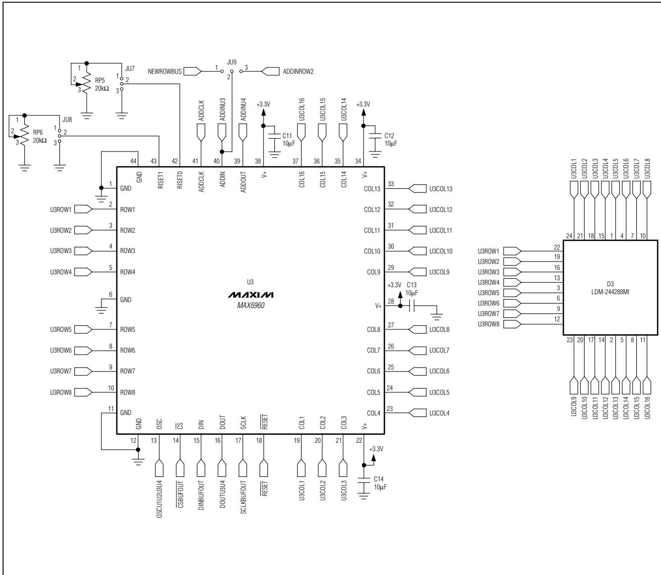
Figure 5. MAX6960 EV Kit Schematic (Sheet 3 of 6)
