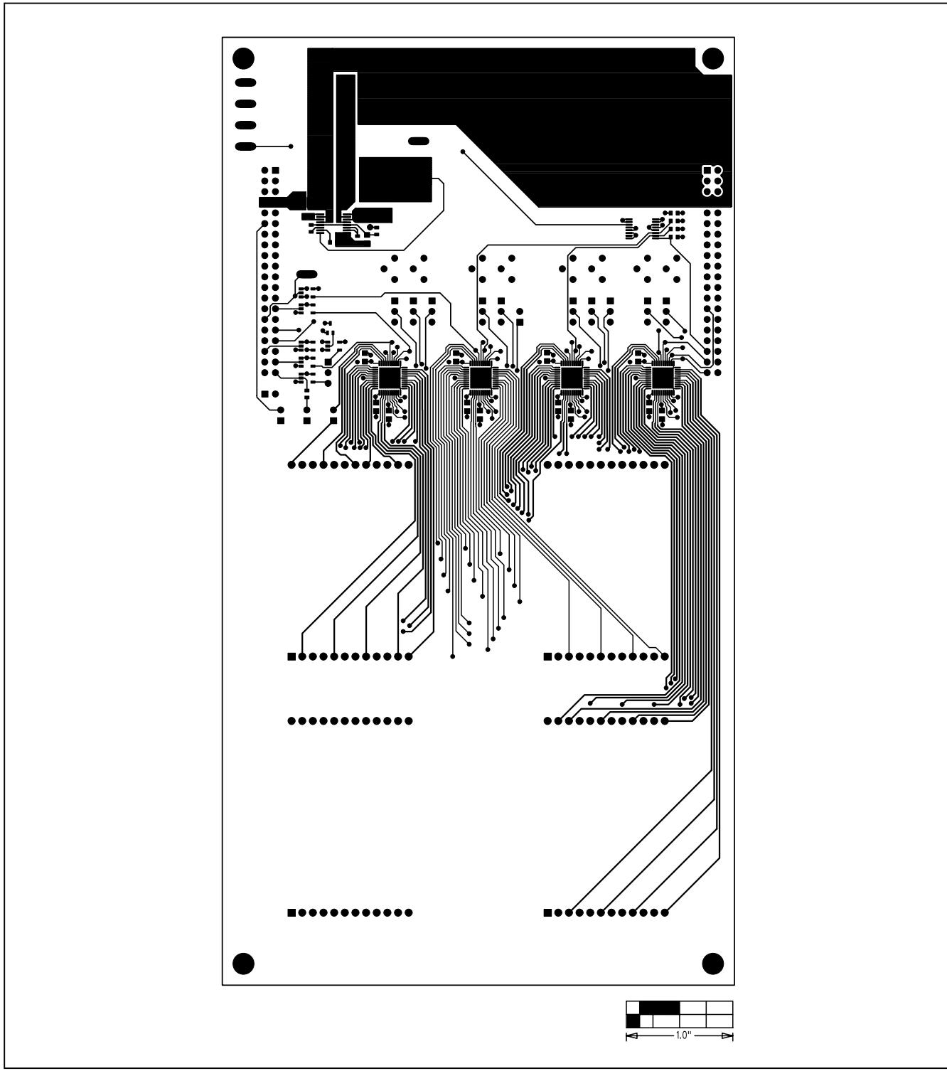
Figure 7. MAX6960 EV Kit PC Board Layout—Component Side
