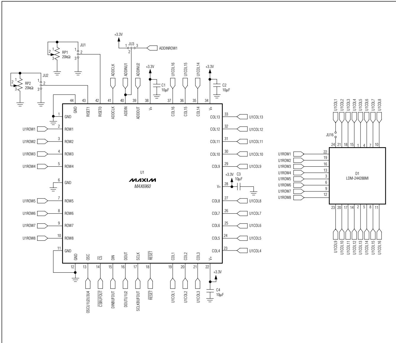
Figure 5. MAX6960 EV Kit Schematic (Sheet 1 of 6)
