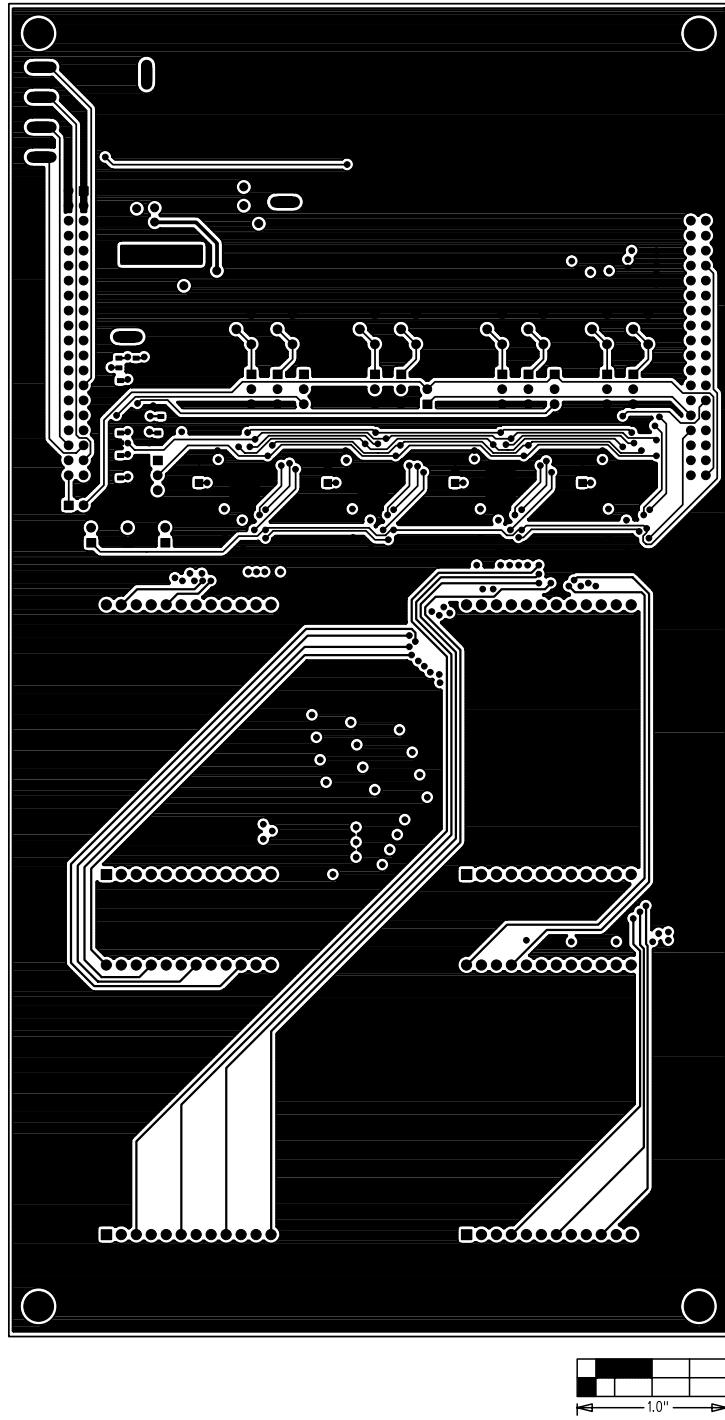
Figure 10. MAX6960 EV Kit PC Board Layout—Solder Side
