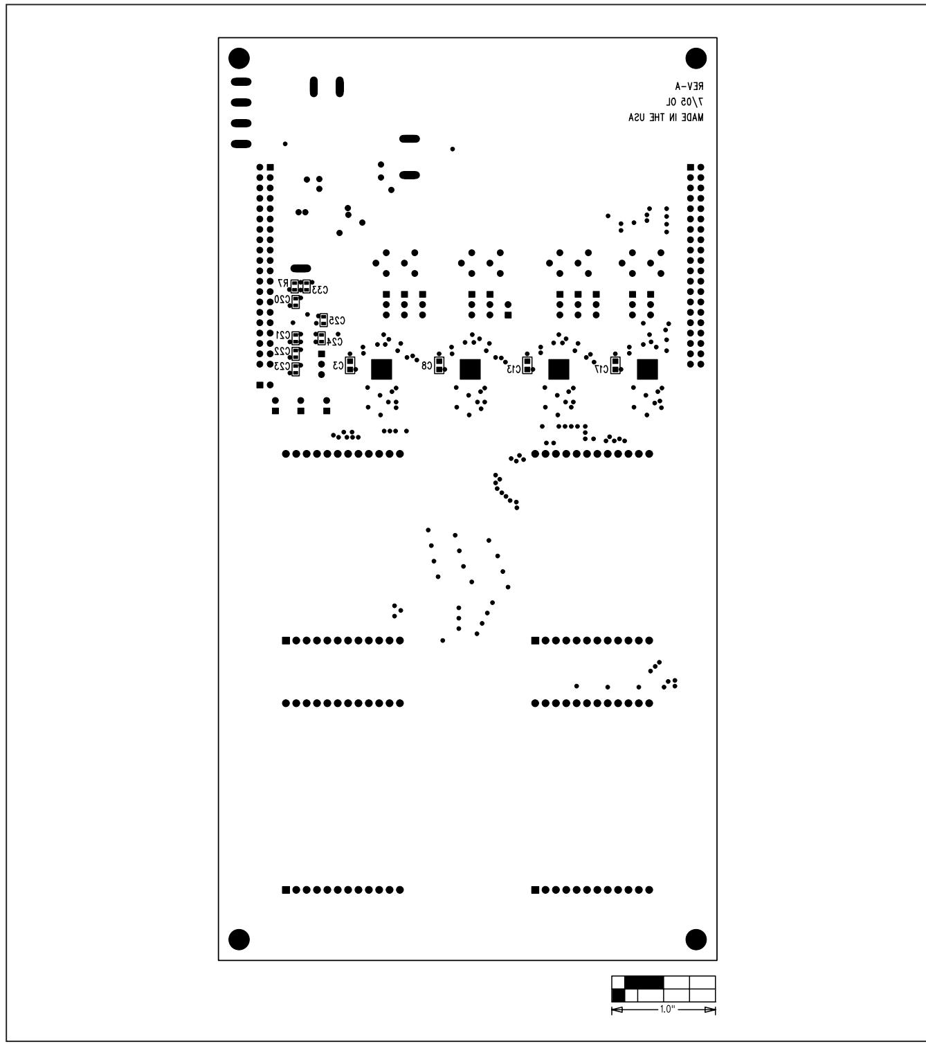
Figure 11. MAX6960 EV Kit Component Placement Guide—Solder Side
