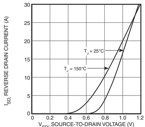
Figure 8, Reverse Drain Current vs Source-to-Drain Voltage
