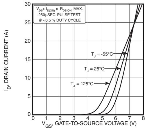
Figure 4, Transfer Characteristics
