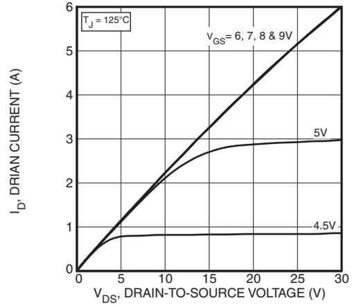
Figure 2, Output Characteristics
