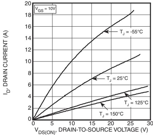
Figure 1, Output Characteristics
