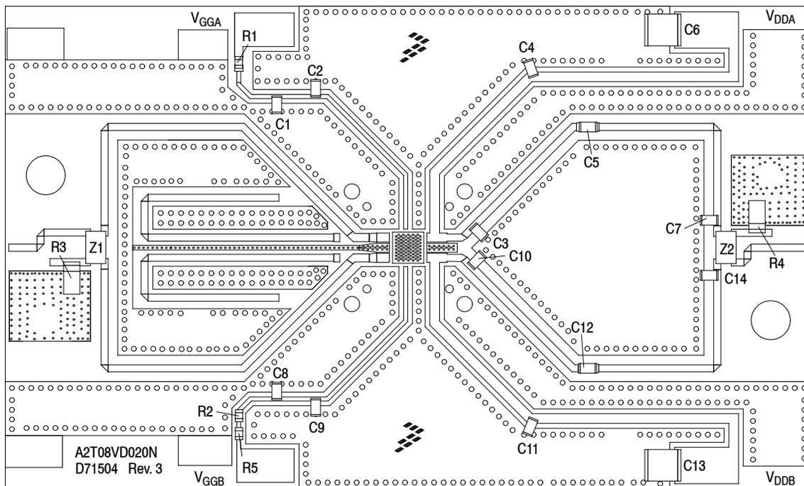
Figure 17. A2T08VD020NT1 Test Circuit Component Layout — 728–768 MHz
