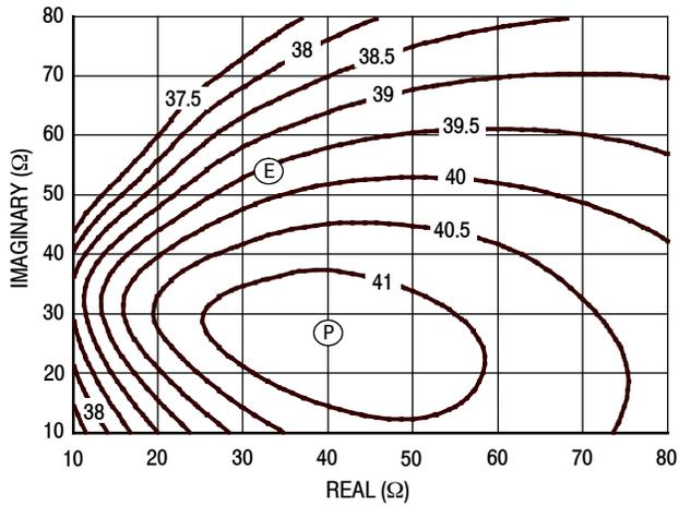
Figure 21. P1dB Load Pull Output Power Contours (dBm)
