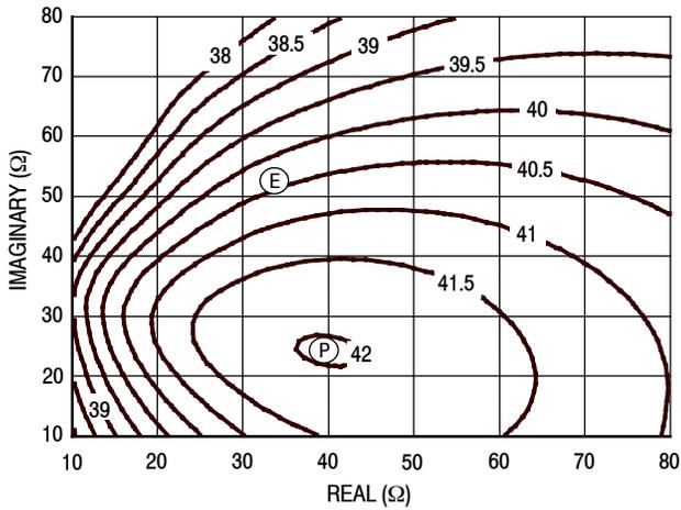
Figure 25. P3dB Load Pull Output Power Contours (dBm)
