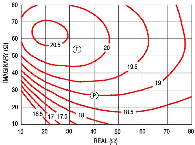
Figure 23. P1dB Load Pull Gain Contours (dB)
