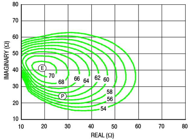
Figure 14. P3dB Load Pull Efficiency Contours (%)
