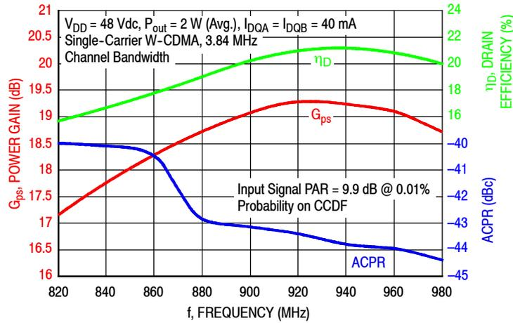
Figure 4. Broadband Performance @  $P_{out} = 2$  Watts Avg.
