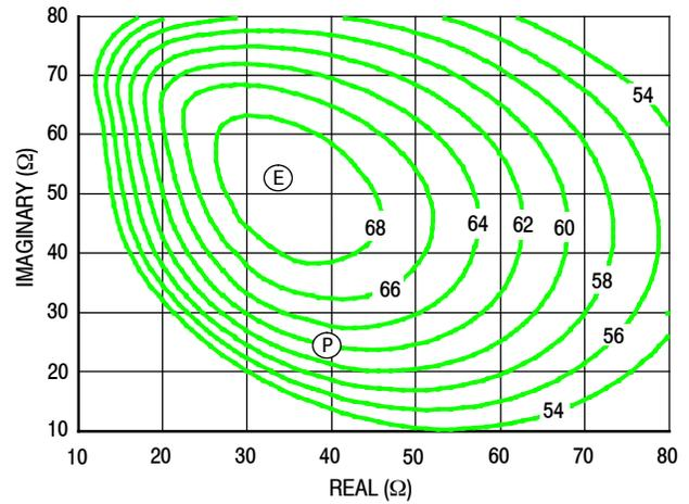
Figure 26. P3dB Load Pull Efficiency Contours (%)
