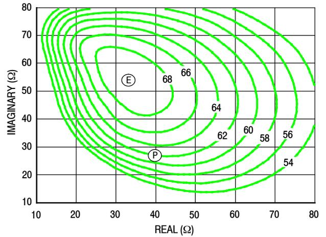
Figure 22. P1dB Load Pull Efficiency Contours (%)
