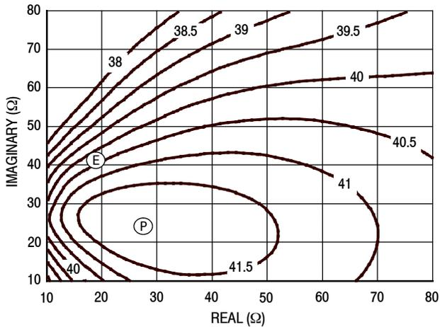
Figure 13. P3dB Load Pull Output Power Contours (dBm)
