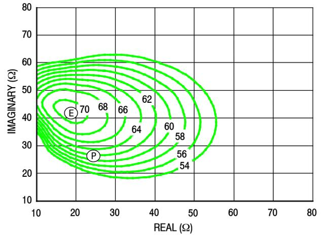
Figure 10. P1dB Load Pull Efficiency Contours (%)
