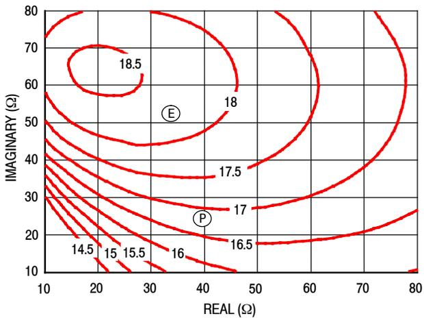
Figure 27. P3dB Load Pull Gain Contours (dB)
