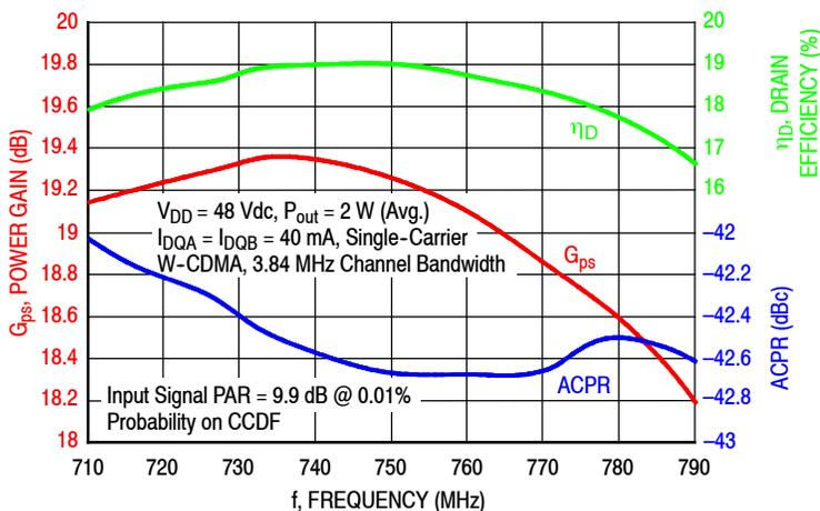
Figure 18. Broadband Performance @  $P_{out} = 2$  Watts Avg.
