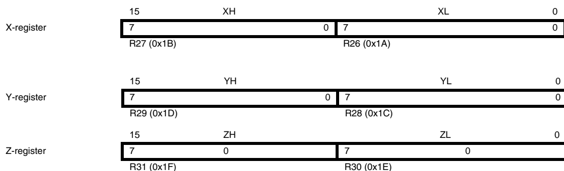
Figure 5-3. The X-, Y-, and Z-registers
