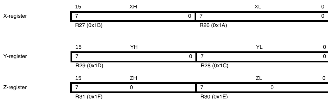
Figure 5-3. The X-, Y-, and Z-registers
