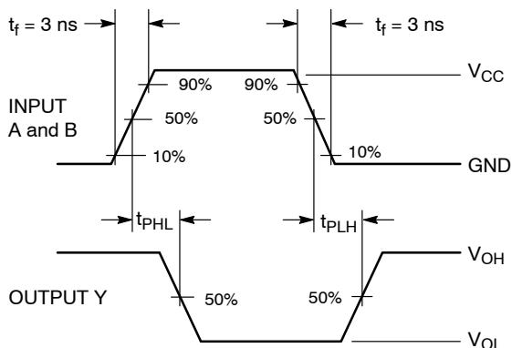
**Figure 3. Switching Waveform**
