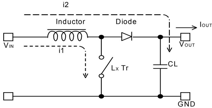
Figure 2. The inductor current (IL) flowing through the inductor (L)
