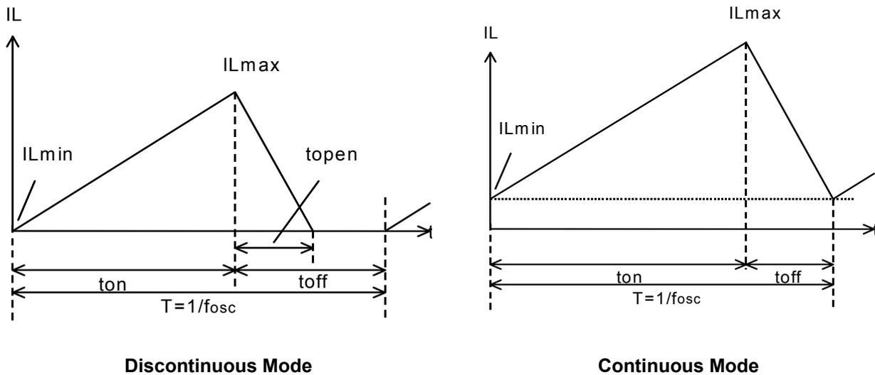
There are two operation modes in the PWM step-up DC/ DC converter: continuous mode and discontinuous mode. When a transistor is in the On-state, the voltage to be applied to L is described as  $V_{IN}$ . An increase in the inductor current ( $i1$ ) can be written as follows:
