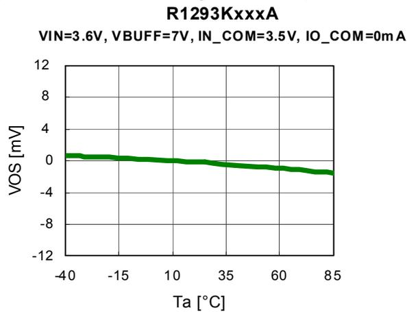
**32) GAMMA Offset Voltage vs. Temperature**
