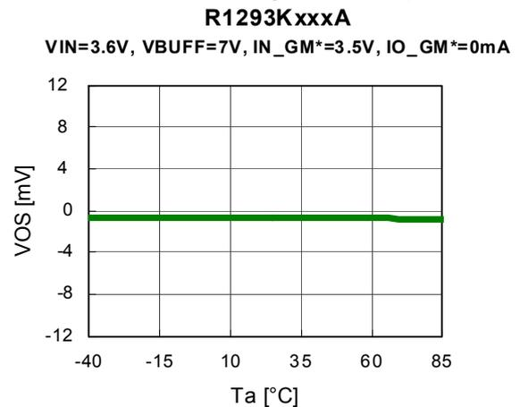
**33) VCOM Output Voltage vs. Temperature**
