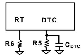
When using Maxduty soft-start, it is recommended that latch protection delay time ( $t_{DLY}$ ) be set  $t_{DLY} > 6 \times (R5 \times C_{DTC})$ .  $t_{DLY}$  should be longer than the soft-start time.
