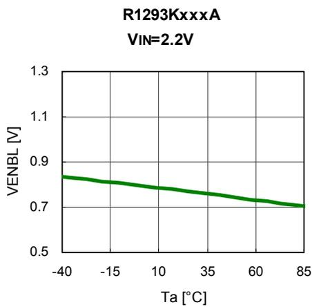
**18) ENB "H" Input Voltage vs. Temperature**
