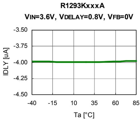
**15) DELAY Pin Discharge Current vs. Temperature**
