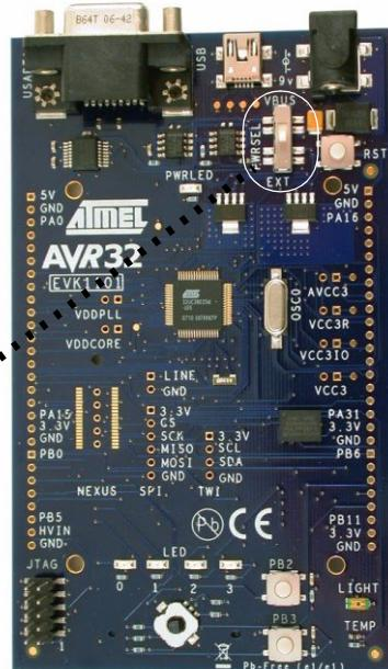
The 4 LEDs shall shortly blink: the Control Panel is up & running.
