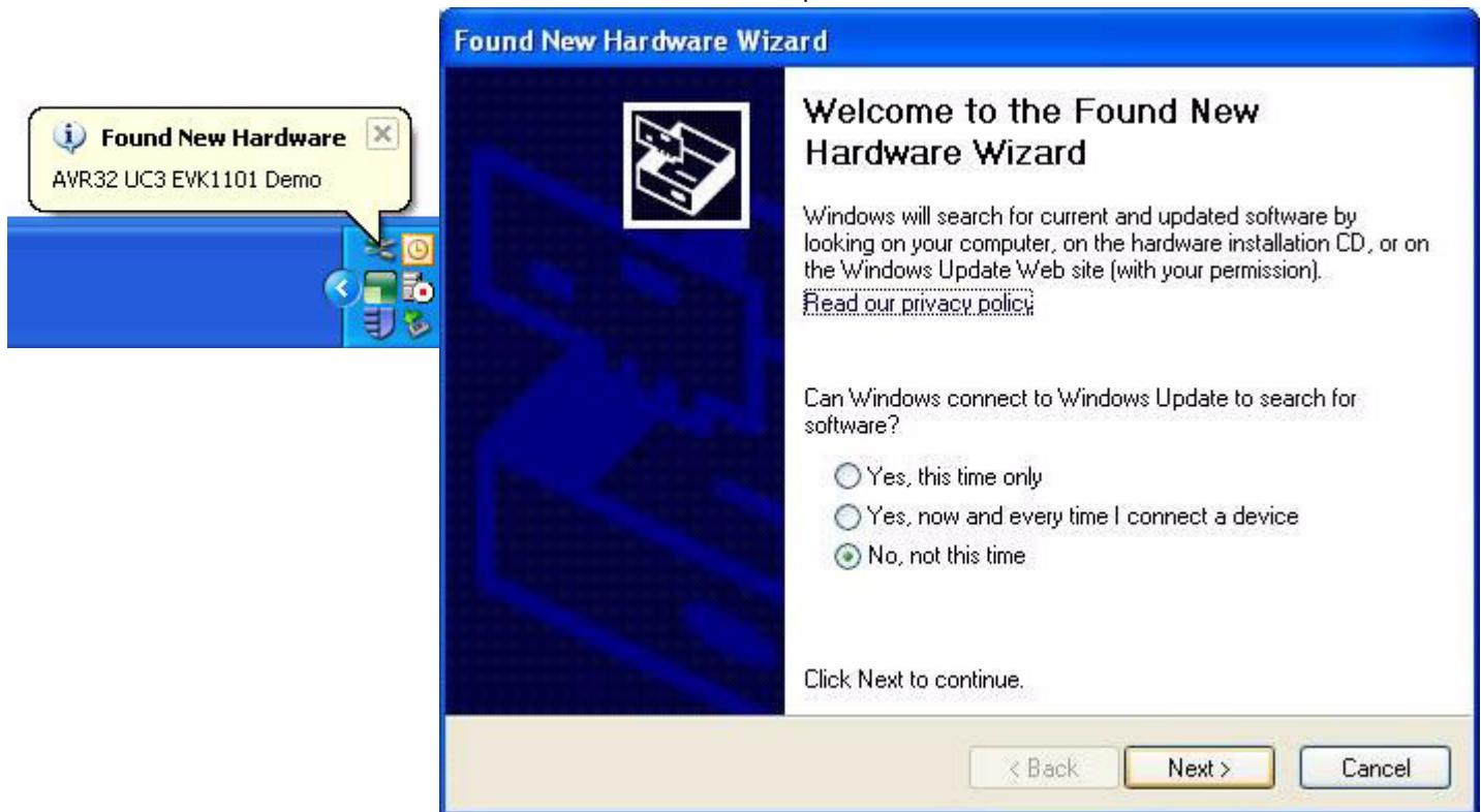
On the next screen, select “Install from a list or specific location (Advanced)” and click ‘Next’. Then request to search in the **usb** folder of the «AVR32 UC3B Control Panel PC Demo» installation directory as shown below and click ‘Next’:
