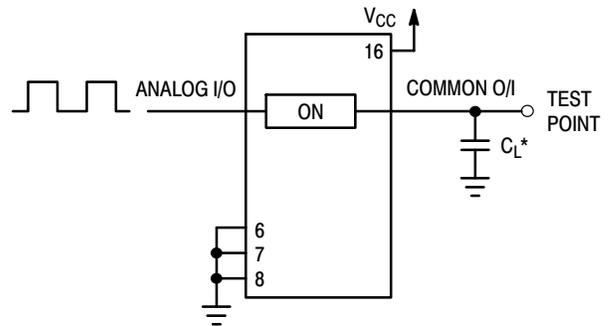
\*Includes all probe and jig capacitance
