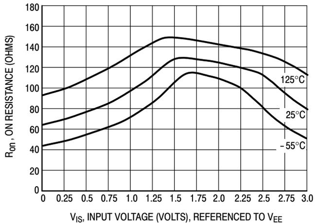
Figure 1b. Typical On Resistance, V<sub>CC</sub> - V<sub>EE</sub> = 3.0 V
