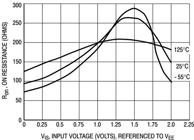
Figure 1a. Typical On Resistance, V<sub>CC</sub> - V<sub>EE</sub> = 2.0 V
