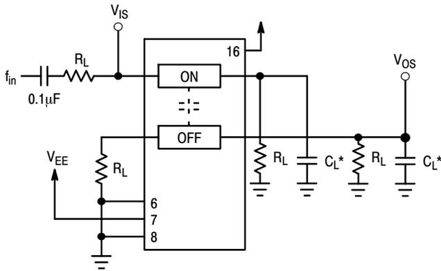
\*Includes all probe and jig capacitance
