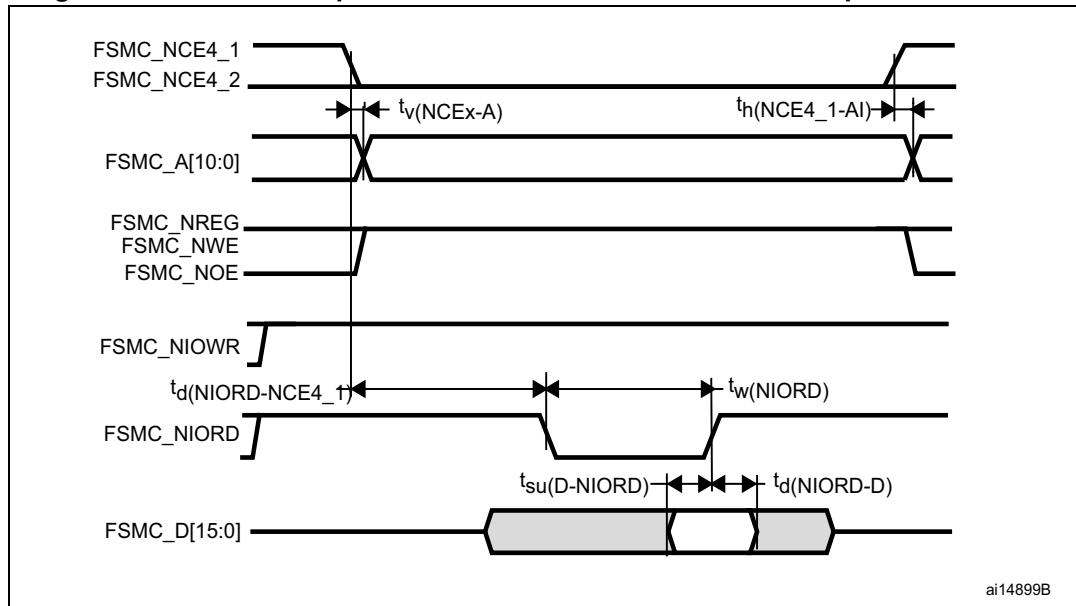
Figure 67. PC Card/CompactFlash controller waveforms for I/O space write access
