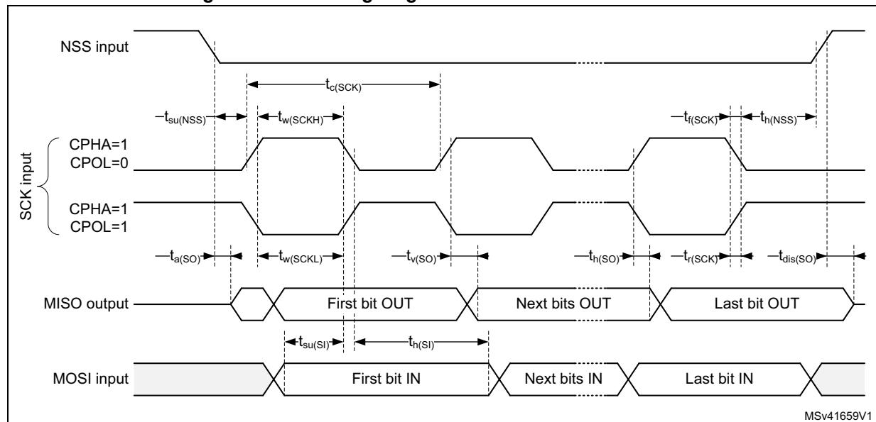
Figure 41. SPI timing diagram - master mode
