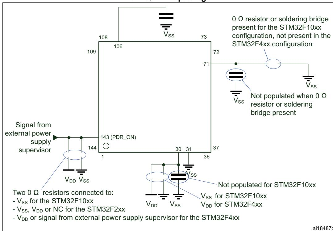
**Figure 4. Compatible board design between STM32F2 and STM32F41xxx
