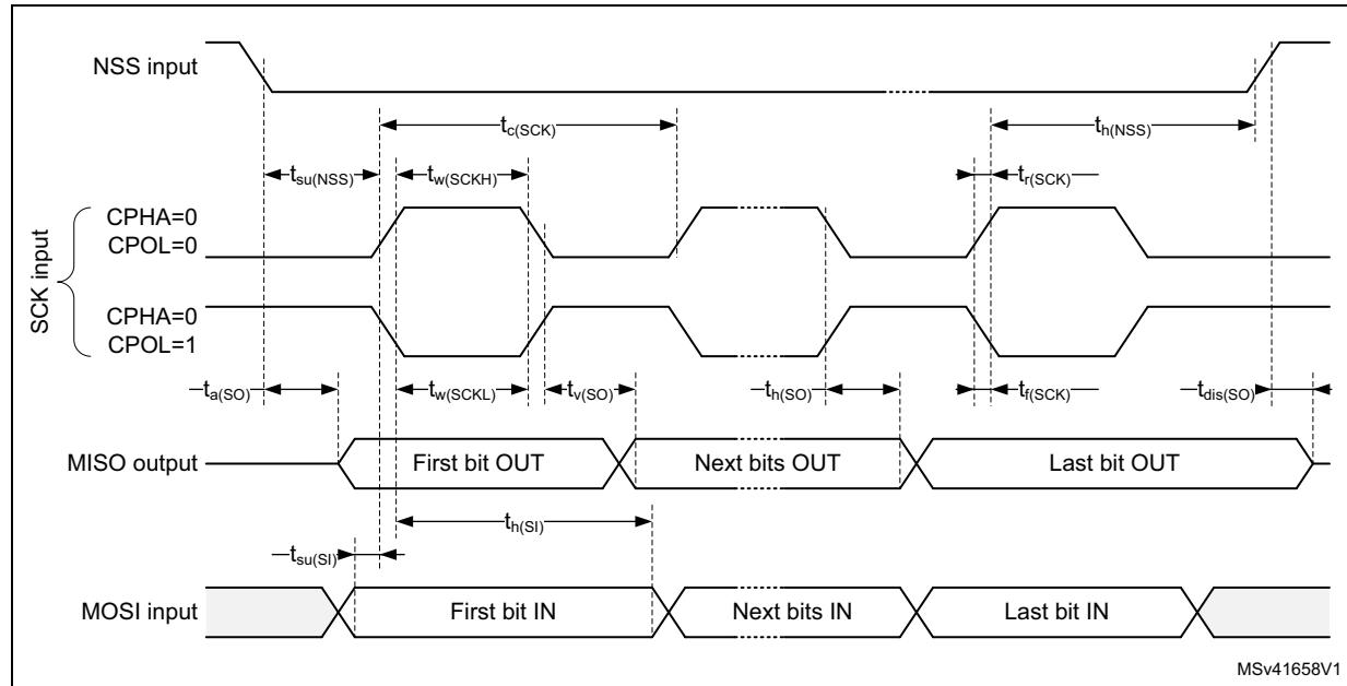
Figure 40. SPI timing diagram - slave mode and CPHA = 1
