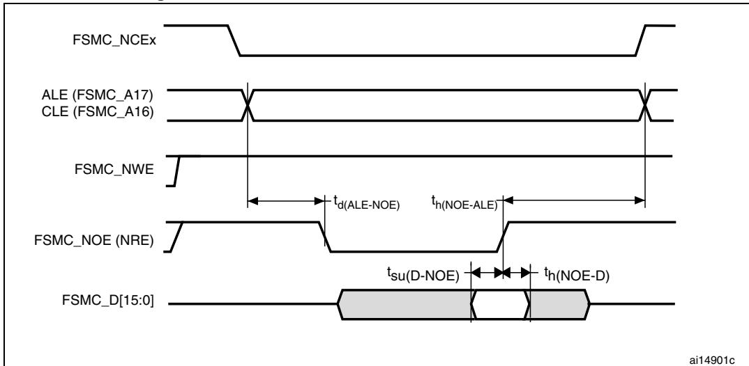
**Figure 69. NAND controller waveforms for write access**
