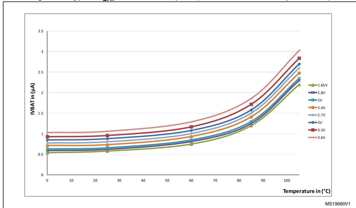
**Figure 29. Typical  $V_{BAT}$  current consumption (LSE and RTC ON/backup RAM ON)**
