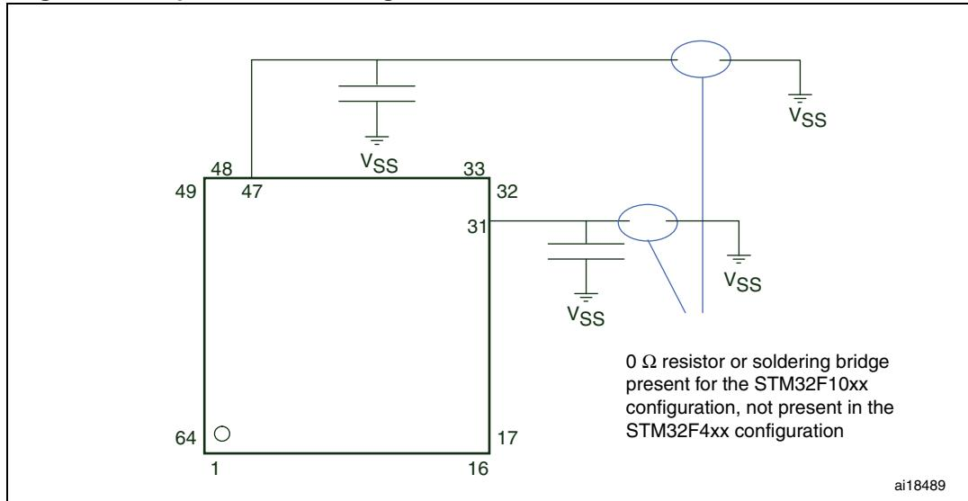
**Figure 2. Compatible board design STM32F10xx/STM32F2/STM32F41xxx for LQFP100 package**
