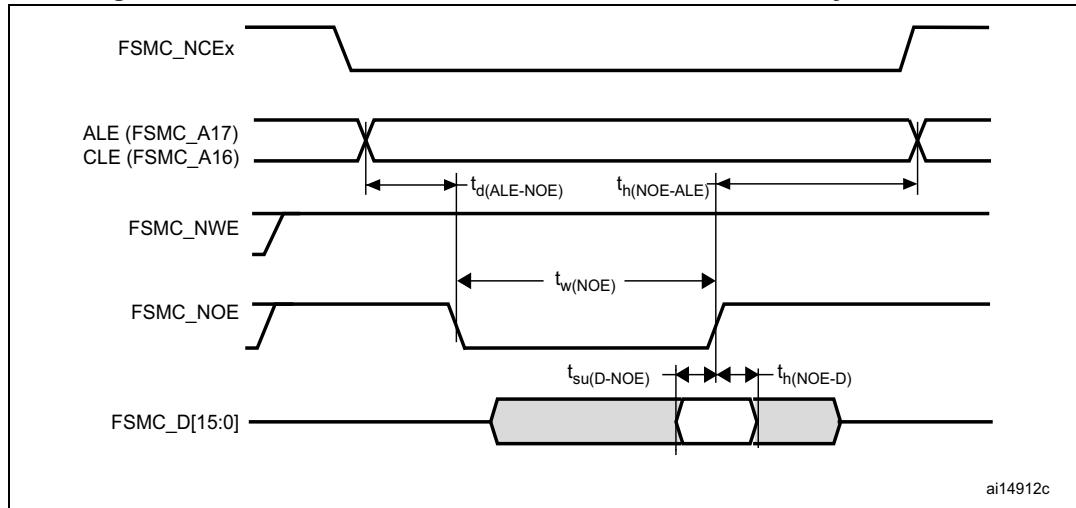
**Figure 71. NAND controller waveforms for common memory write access**
