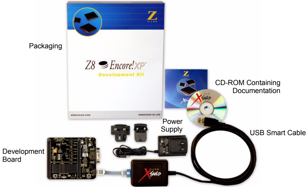
Figure 1. Z8 Encore! XP® 4K Series 8-Pin Development Kit Contents (Printed Quick Start Guide Not Shown)
