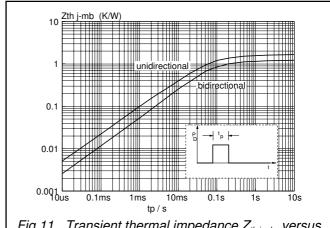
Fig.11. Transient thermal impedance  $Z_{th j-mb}$ , versus pulse width t<sub>o</sub>.
