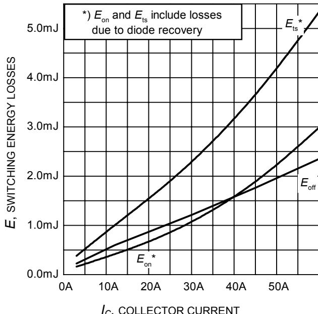
**Figure 13. Typical switching energy losses as a function of collector current**
