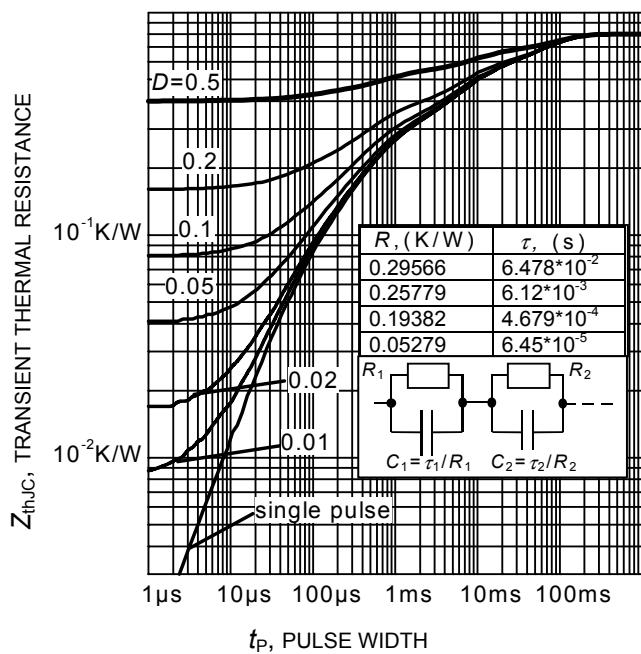
**Figure 21. IGBT transient thermal resistance**
