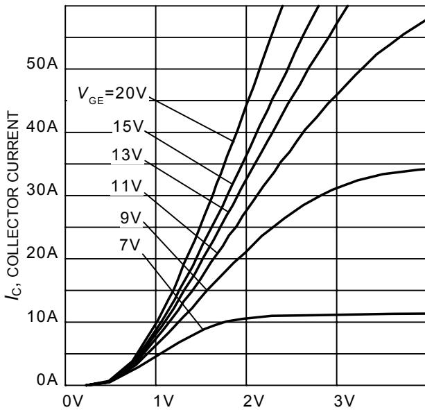
**Figure 6. Typical output characteristic**
