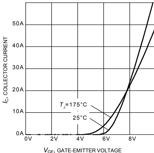
**Figure 7. Typical transfer characteristic**
