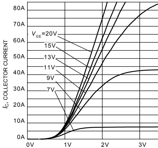
**Figure 5. Typical output characteristic**
