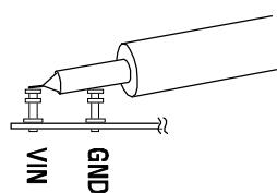
Figure 2. Measuring Input or Output Ripple
