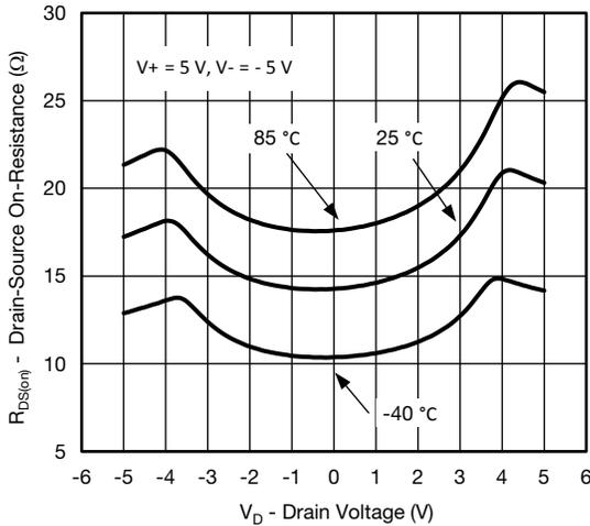
**R<sub>DS(on)</sub> vs. V<sub>D</sub> and Temperature (Dual Supply)**
