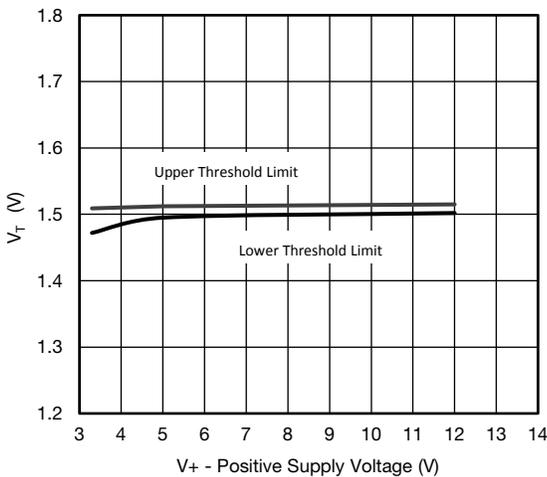
**Input Threshold vs. V<sub>+</sub> Supply Voltage**
