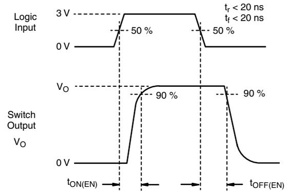
Fig. 3 - Enable Switching Time
