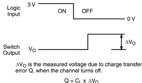
**Fig. 5 - Charge Injection**
