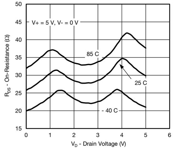
**R<sub>DS(on)</sub> vs. V<sub>D</sub> and Temperature**
