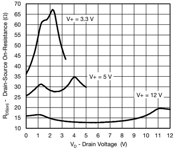
**R<sub>DS(on)</sub> vs. V<sub>D</sub> and Power Supply**
