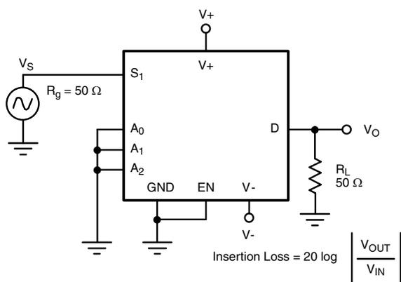
**Fig. 8 - Insertion Loss**
