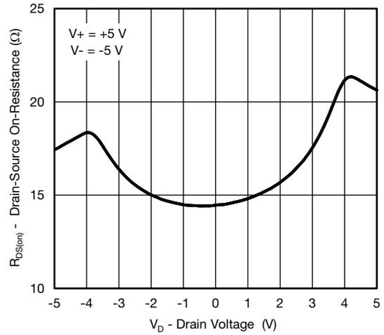
**R<sub>DS(on)</sub> vs. V<sub>D</sub> and Power Supply**
