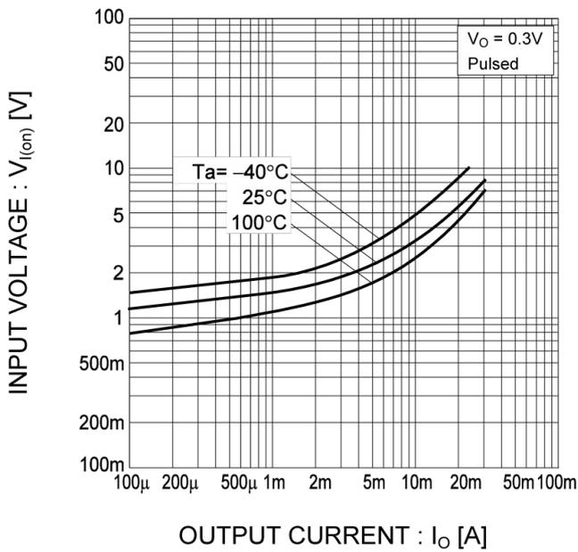
Fig.2 Output Current vs. Input Voltage
