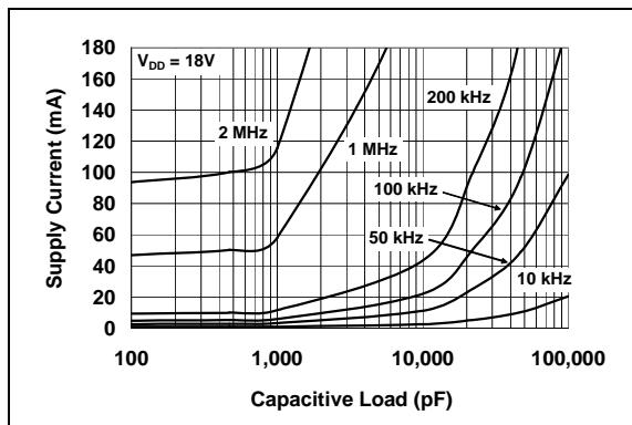
**FIGURE 2-16:** Supply Current vs. Capacitive Load ( $V_{DD} = 18\text{V}$ ).
