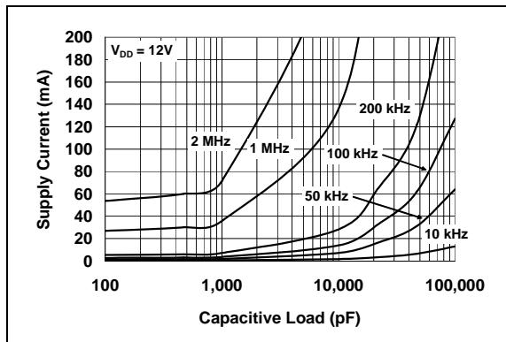
**FIGURE 2-17:** Supply Current vs. Capacitive Load ( $V_{DD} = 12\text{V}$ ).
