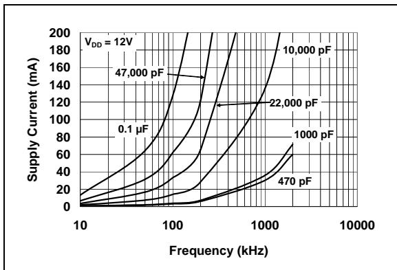
**FIGURE 2-20:** Supply Current vs. Frequency ( $V_{DD} = 12\text{V}$ ).
