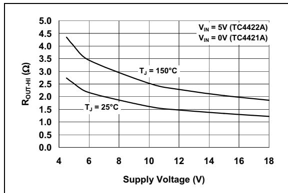
**FIGURE 2-14:** High-State Output Resistance vs. Supply Voltage.
