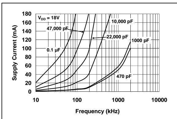
**FIGURE 2-19:** Supply Current vs. Frequency ( $V_{DD} = 18\text{V}$ ).
