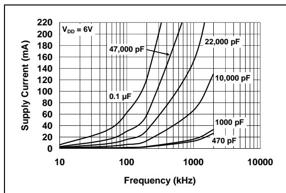
**FIGURE 2-21:** Supply Current vs. Frequency ( $V_{DD} = 6\text{V}$ ).
