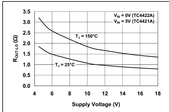
**FIGURE 2-15:** Low-State Output Resistance vs. Supply Voltage.
