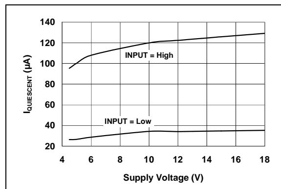
**FIGURE 2-10:** Quiescent Supply Current vs. Supply Voltage.
