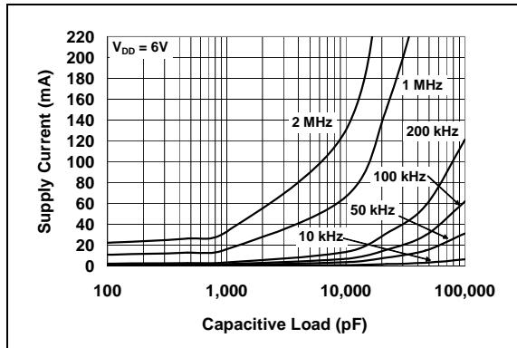
**FIGURE 2-18:** Supply Current vs. Capacitive Load ( $V_{DD} = 6\text{V}$ ).
