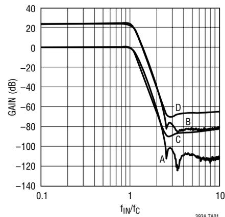
A:  $f_C = 10\text{kHz}$ , GAIN = 1,  $V_{IN} = 1\text{VRMS}$
