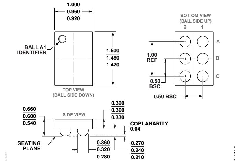
Figure 17. 6-Ball Wafer Level Chip Scale Package [WLCSP]
