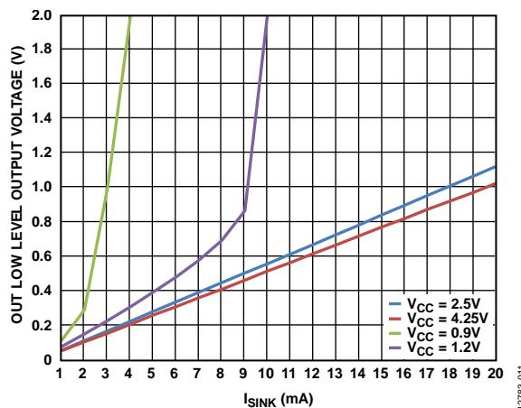
Figure 11. OUT Low Level Output Voltage ( $V_{OUT\_OU}$ ) vs. Sink Current ( $I_{SINK}$ )
