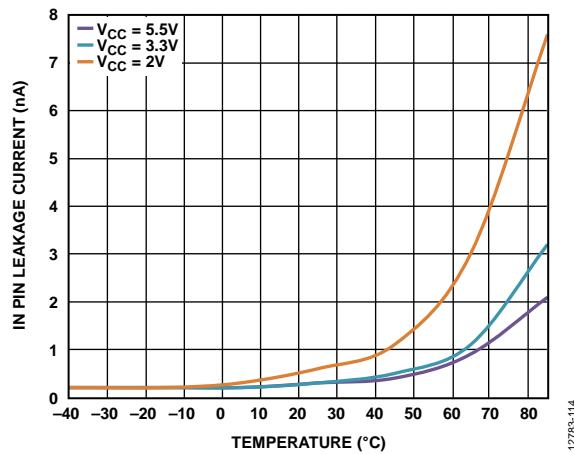
Figure 9. IN Pin Leakage Current vs. Temperature
