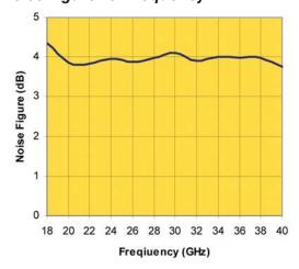
Note: Measured Performance Characteristics (Typical Performance at 25°C) Vd1 = 5V, Id1 = 45 mA
