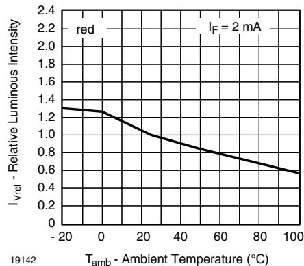
Figure 17. Relative Luminous Intensity vs. Amb. Temperature
