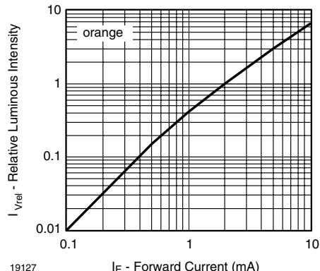
Figure 1. Relative Luminous Intensity vs. Forward Current
