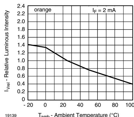
Figure 5. Relative Luminous Intensity vs. Amb. Temperature
