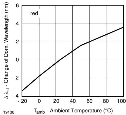
Figure 16. Change of Dominant Wavelength vs. Ambient Temperature
