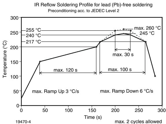
Figure 19. Vishay Lead (Pb)-free Reflow Soldering Profile
