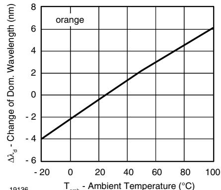
Figure 4. Change of Dominant Wavelength vs. Ambient Temperature
