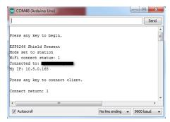
Once you get to the final, server example of the sketch, try loading up a web browser and navigating to the displayed web address. The ESP8266 should serve up a web page like this:
