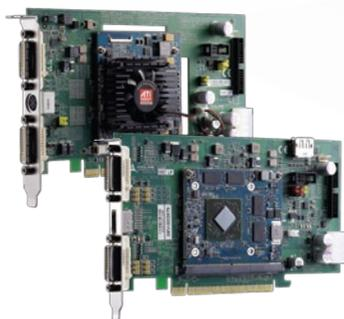
ADLINK's PCIe x16 MXM carrier boards allow for discrete PCIe graphics expansion using a Mobile PCI Express Module (MXM). The MXM carrier board series supports MXM-II and MXM-III graphics modules, allowing developers to evaluate, prototype and verify MXM graphics modules before full integration into the custom carrier board design.
