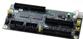
The Flat Panel Transfer Board (FPTB) supports prototyping and verification of LVDS and TTL flat panel displays with Express-BASE and nanoX-BASE carrier boards and is equipped with an LVDS-to-TTL converter to allow users to implement TTL displays with COM Express systems that support LVDS only. Onboard PWM circuitry supports backlight control for LVDS and TTL displays.
