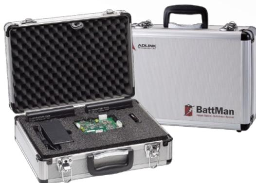
The BattMan Smart Battery Management Reference System supports two Smart Batteries and provides ATX power for COM Express mobile embedded systems. The BattMan system allows developers to easily implement battery power in COM Express based applications requiring high mobility.
