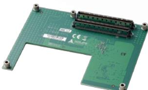
The COM-T6T2 adapter board allows COM Express Type 6 modules to be backwards compatible with Type 2 carrier boards. A SATA-to-PATA converter and PCIe-to-PCI bridge are onboard to provide signal conversion to the required COM Express Type 2 interfaces. The SDVO port is rerouted to correspond with the Type 2 pin definition (no PCIe x16).
