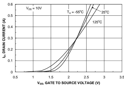
**Figure 5. Transfer Characteristics.**
