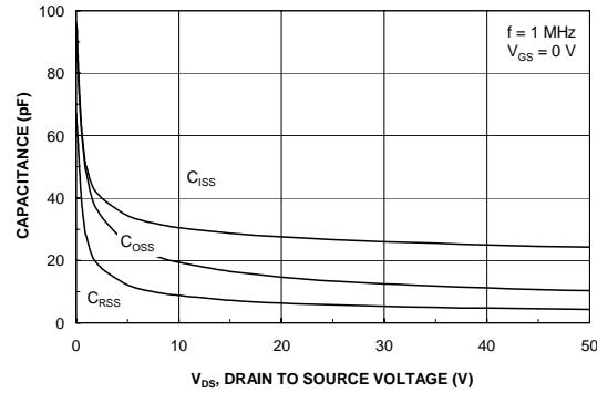
**Figure 8. Capacitance Characteristics.**
