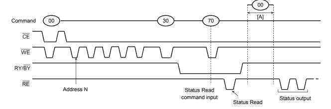
The device status can be read out by inputting the Status Read command "70h" in Read mode. Once the device has been set to Status Read mode by a "70h" command, the device will not return to Read mode unless the Read command "00h" is input during [A]. If the Read command "00h" is input during [A], Status Read mode is reset, and the device returns to Read mode. In this case, data output starts automatically from address N and address input is unnecessary.
