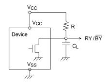
This data may vary from device to device. We recommend that you use this data as a reference when selecting a resistor value.
