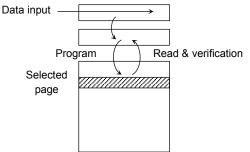
The data is transferred (programmed) from the Data Cache via the Page Buffer to the selected page on the rising edge of  $\overline{\text{WE}}$  following input of the "10h" command. After programming, the programmed data is transferred back to the Page Buffer to be automatically verified by the device. If the programming does not succeed, the Program/Verify operation is repeated by the device until success is achieved or until the maximum loop number set in the device is reached.
