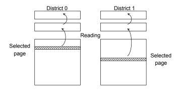
The data transfer operation from the cell array to the Data Cache via Page Buffer starts on the rising edge of  $\overline{\text{WE}}$  in the 30h command input cycle (after the 2 Districts address information has been latched). The device will be in the Busy state during this transfer period.
