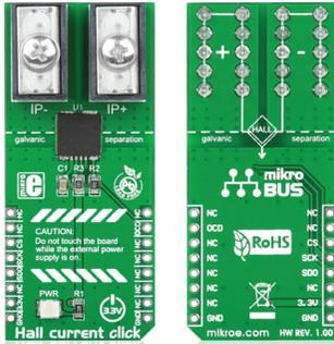
Hall current click™ is a high precision current sensor. It carries a galvanically isolated TL14970-D050T4 miniature magnetic digital current sensor that utilizes the Hall effect to measure electric current. The board carries two EXtreme ZPower connectors to connect the conductor. The sensor readings are sent to the target board through the mikroBUS™ SPI (SDO, SCK, and CS) lines. The board uses a 3.3V power supply only.
