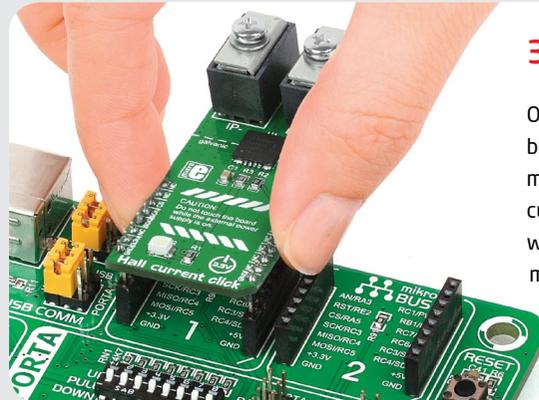
Once you have soldered the headers your board is ready to be placed into the desired mikroBUS™ socket. Make sure to align the cut in the lower-right part of the board with the markings on the silkscreen at the mikroBUS™ socket. If all the pins are aligned correctly, push the board all the way into the socket.
