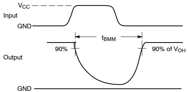
**Figure 2.**  $t_{BBM}$  (Time Break-Before-Make)
