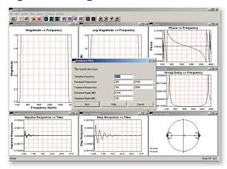
The Digital Filter Design Tool makes designing and analyzing FIR and IIR filters easy. Enter frequency specifications and filter code and coefficients are generated automatically. Graphical output windows provide the desired filter's characteristics.
