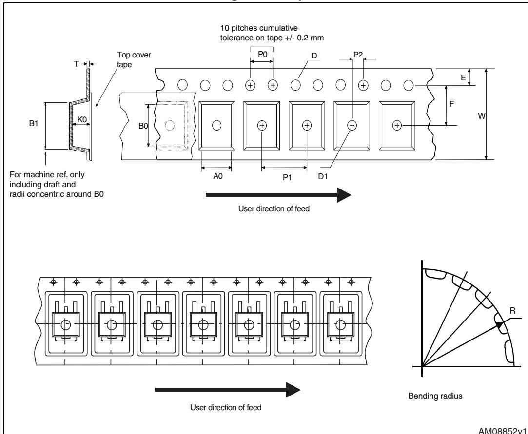
**Table 12. D<sup>2</sup>PAK (TO-263) tape and reel mechanical data**
