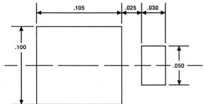
Figure 1. Suggested Mounting Pad Dimensions
