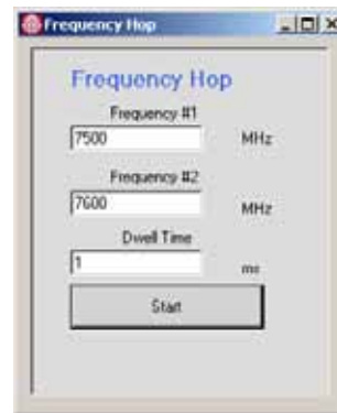
Figure 17. Typical Setting Example of Frequency Hop
