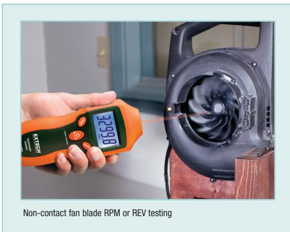
Non-contact fan blade RPM or REV testing
