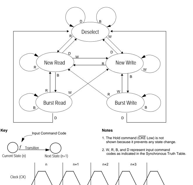
Current State and Next State Definition for Pipelined and Flow Through Read/Write Control State Diagram
