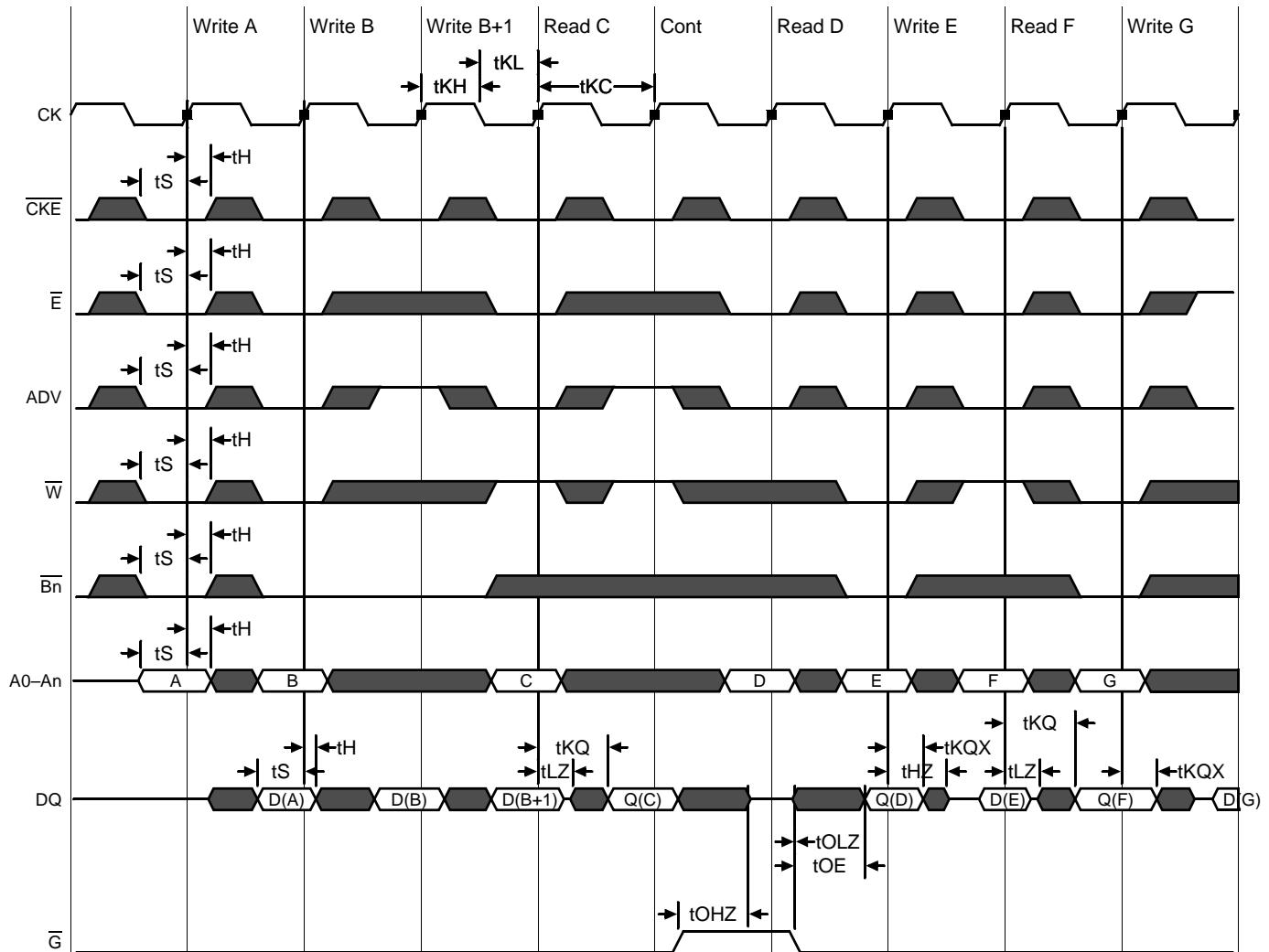
\*Note:  $\overline{E} = \text{High}(\text{False})$  if  $\overline{E1} = 1$  or  $E2 = 0$  or  $\overline{E3} = 1$
