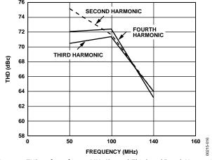
Figure 16. THD vs.  $f_{CLK} @ f_{OUT} = 2 MHz$  (Second, Third, and Fourth Harmonics)
