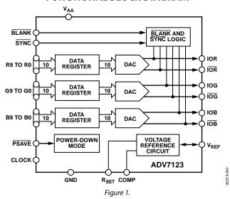
The ADV7123 is fabricated in a 5 V CMOS process. Its monolithic CMOS construction ensures greater functionality with lower power dissipation. The ADV7123 is available in a 48-lead LQFP package.
