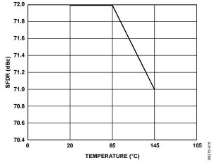
Figure 15. SFDR vs. Temperature @  $f_{CLK} = 50$  MHz,  $(f_{OUT} = 1$  MHz)
