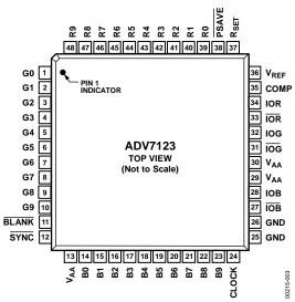
Figure 3. Pin Configuration
