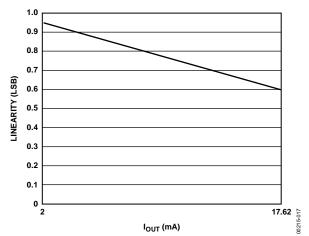
Figure 17. Linearity vs. IOUT
