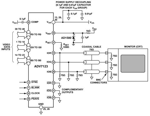
Figure 28. Typical Connection Diagram
