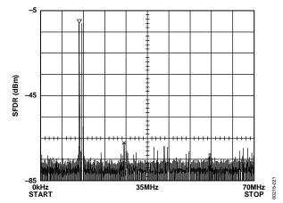
Figure 21. Dual-Tone SFDR @  $f_{CLK} = 140$  MHz ( $f_{OUT1} = 13.5$  MHz,  $f_{OUT2} = 14.5$  MHz)
