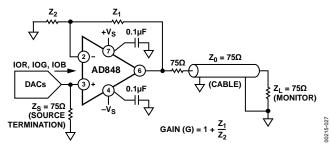
Figure 27. AD848 As an Output Buffer
