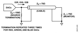
Figure 25. Analog Output Termination for RS-170
