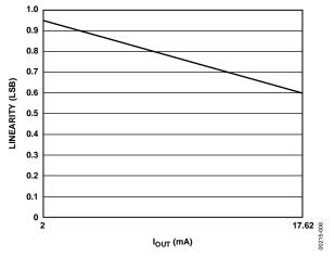
Figure 8. Linearity vs. IOUT
