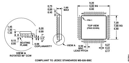
Figure 29. 48-Lead Low Profile Quad Flat Package [LQFP] (ST-48) Dimensions shown in millimeters
