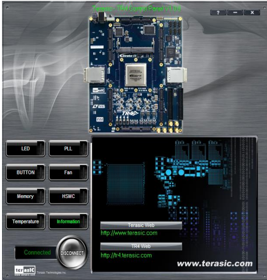
Figure 3-13 Information Tab of TR4 Control Panel
