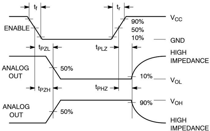
Figure 16. Propagation Delays, Enable to Analog Out
