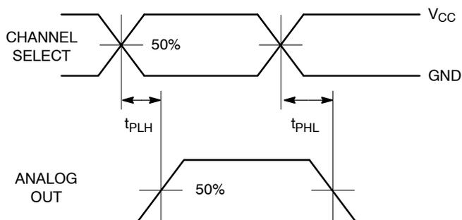
Figure 14. Propagation Delays, Channel Select to Analog Out
