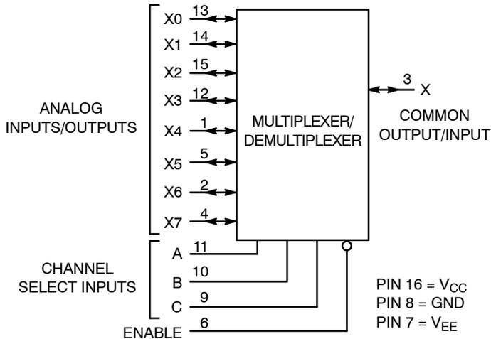
**Figure 2. Logic Diagram**
