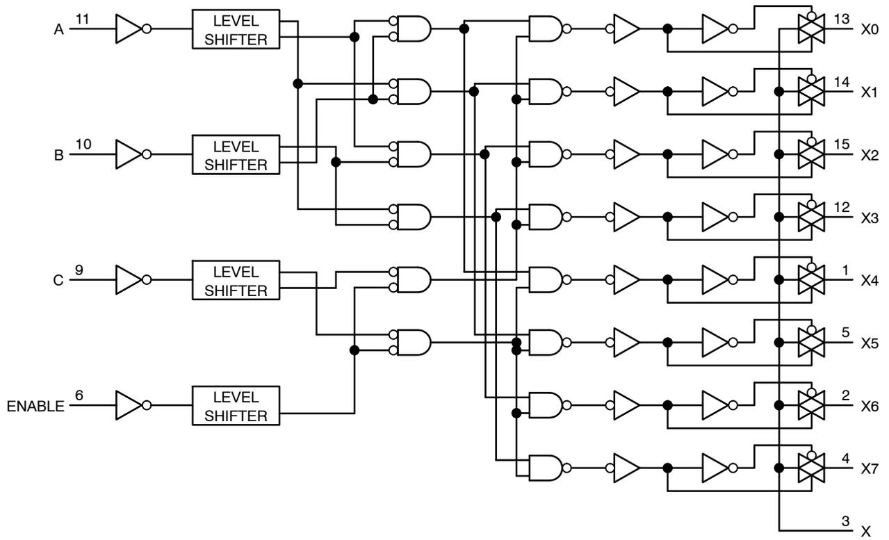
Figure 23. Function Diagram, LVX4051
