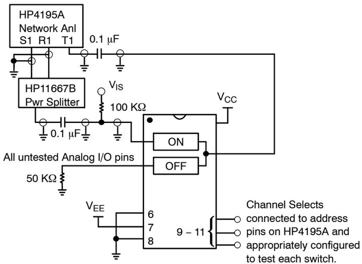
Figure 7. Maximum On Channel Bandwidth, Test Set-Up
