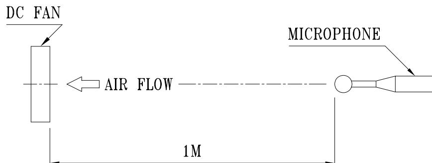
NOISE IS MEASURED AT RATED VOLTAGE IN FREE AIR IN ANECHOIC
