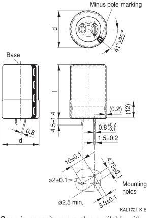
Snap-in capacitors are also available with 3 terminals (length (4.5-1.4) mm). PET insulation cap is positioned under the
