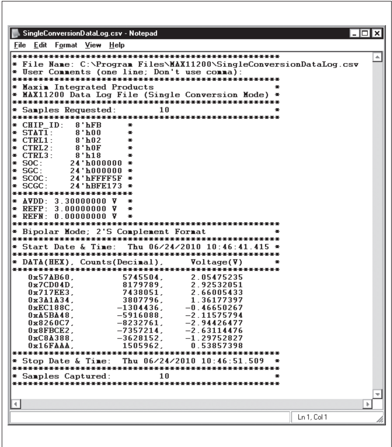
Figure 7. MAX11200/MAX11206/MAX11209/MAX11210/MAX11213 EV Kit Software (Logged Data Opened in Notepad)
