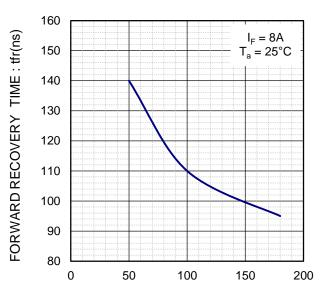
RATE OF CHANGE OF CURRENT :  $di/dt(A/\mu s)$  di/dt-tfr CHARACTERISTICS
